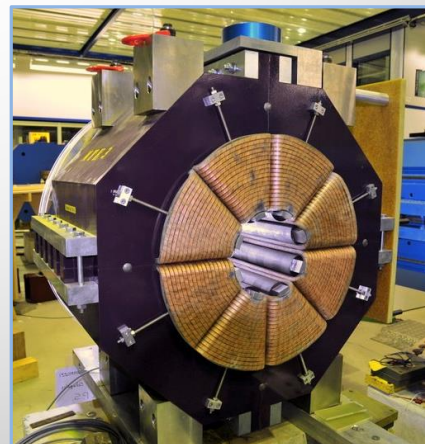
PS Multi-turn extraction octupole
