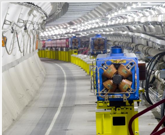
CNGS transfer-line quadrupoles
