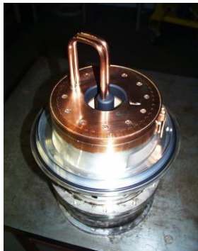
Main coupler PSI cyclotron
