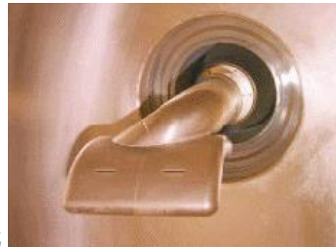
Capacitive coupler of CERN PS 40 MHz
