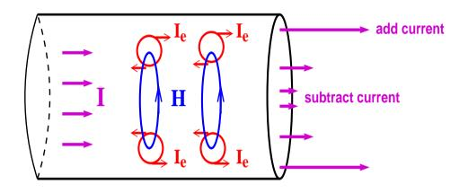
Eddy currents  $I_E$  from changing  $\vec{H}$ -field:  $\nabla \times \vec{E} = \mu_0 \frac{d\vec{H}}{dt}$ Cancel current flow in the centre of the conductor  $I - I_e$ Enforce current flow near the "skin" (surface)  $I + I_e$ Q: Why are high frequency cables thin ??
