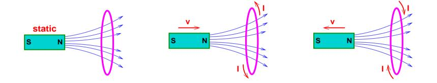
Moving the magnet changes the flux:  $\underline{more}$  or  $\underline{fewer}$  passing through the area (use a conducting coil, e.g. wedding ring)  $\Longrightarrow$
