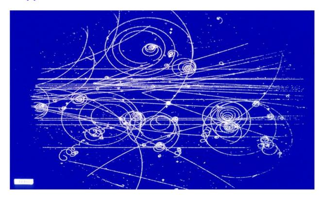
Tracks from particle collisions, lower energy particles have smaller bending radius, allows determination of momenta ..
