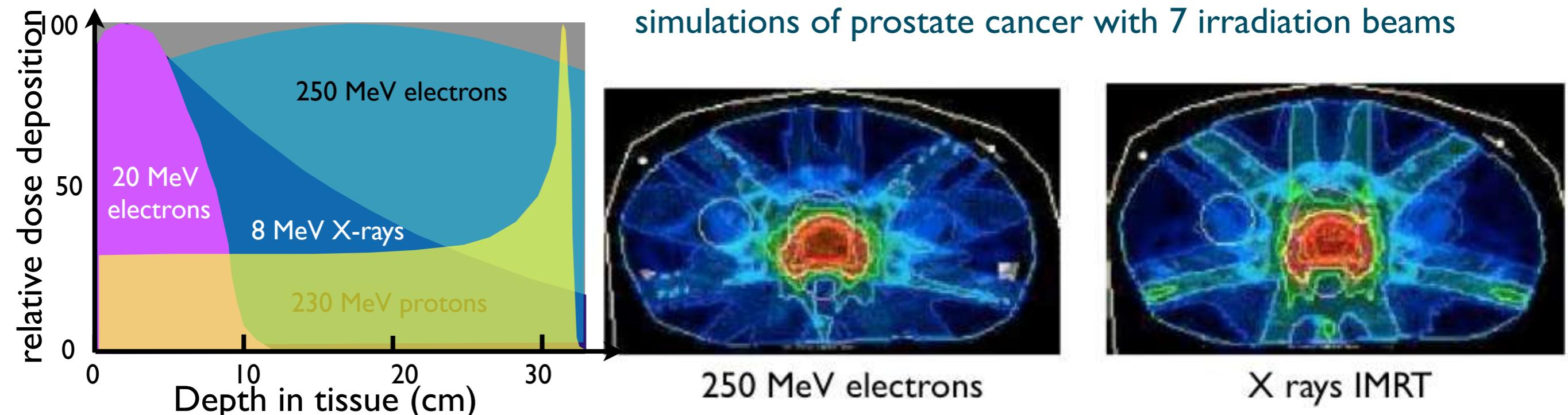
A comparison of dose deposition with 6 MeV X ray an improvement of the quality of a clinically approved prostate treatment plan. While the target coverage is the same or even slightly better for 250 MeV electrons compared to photons the dose sparing of sensitive structures is improved (up to 19%).
