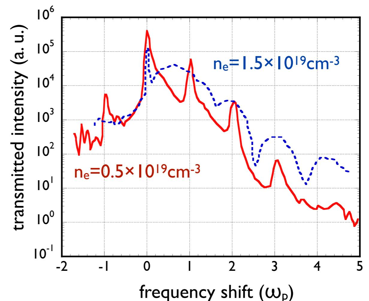
Multiple satellites : high amplitude plasma waves
