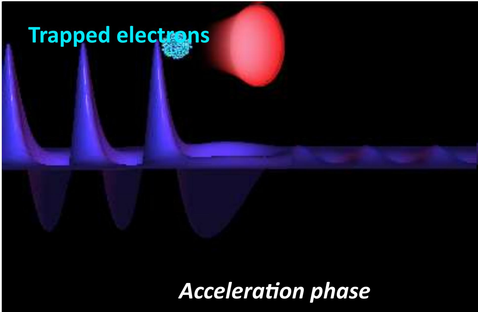
The first laser creates the accelerating structure
