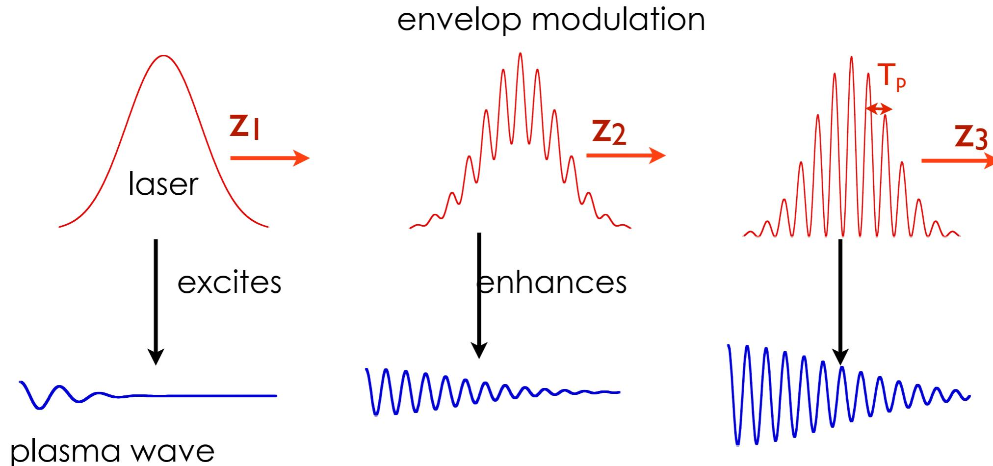
$P_L > P_c(\text{GW}) = 17 n_c/n_e$  then wavebreaking can occur
