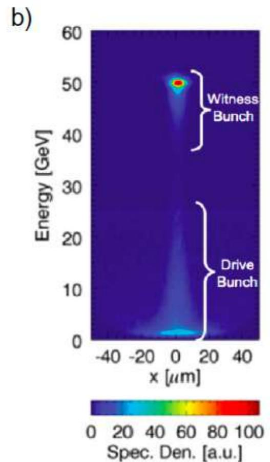
The energy gain is almost linear up to a distance of 65 cm. At 80 cm, the 25 GeV witness bunch has doubled in energy with an 3% energy spread.
