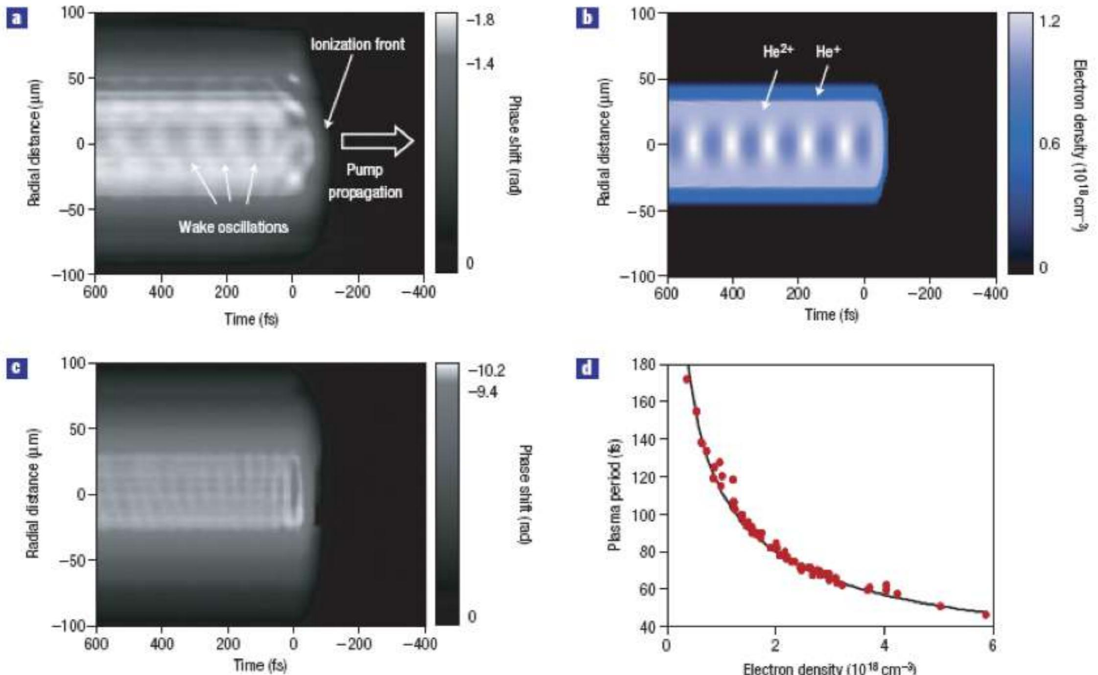
Small amplitude wakes with flats wavefronts. a) probe phase shift 10TW, 30 fs at  $0.95 \times 10^{19} \text{ cm}^{-3}$ .
