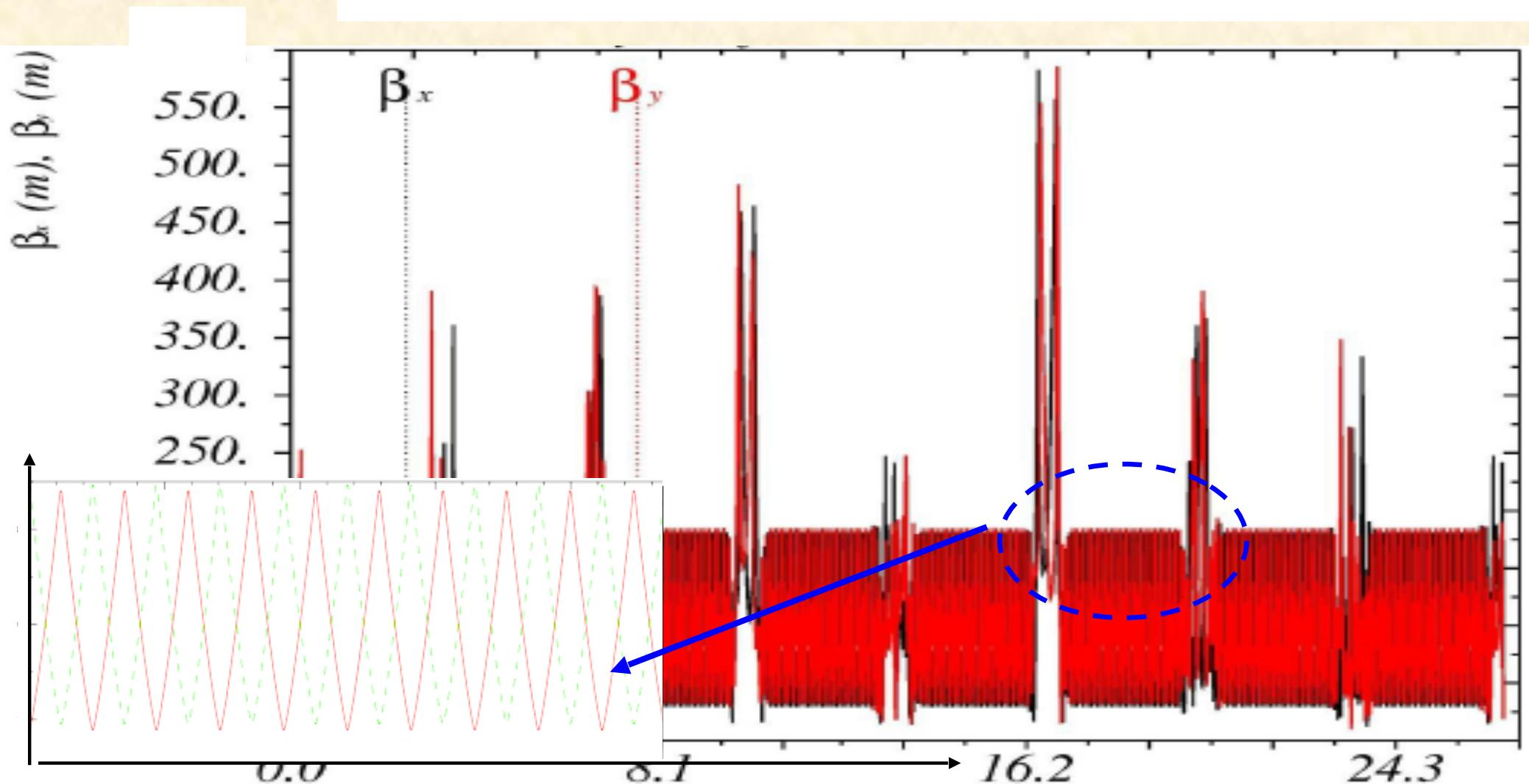
Starting point for the calculation: in the middle of a focusing quadrupole
