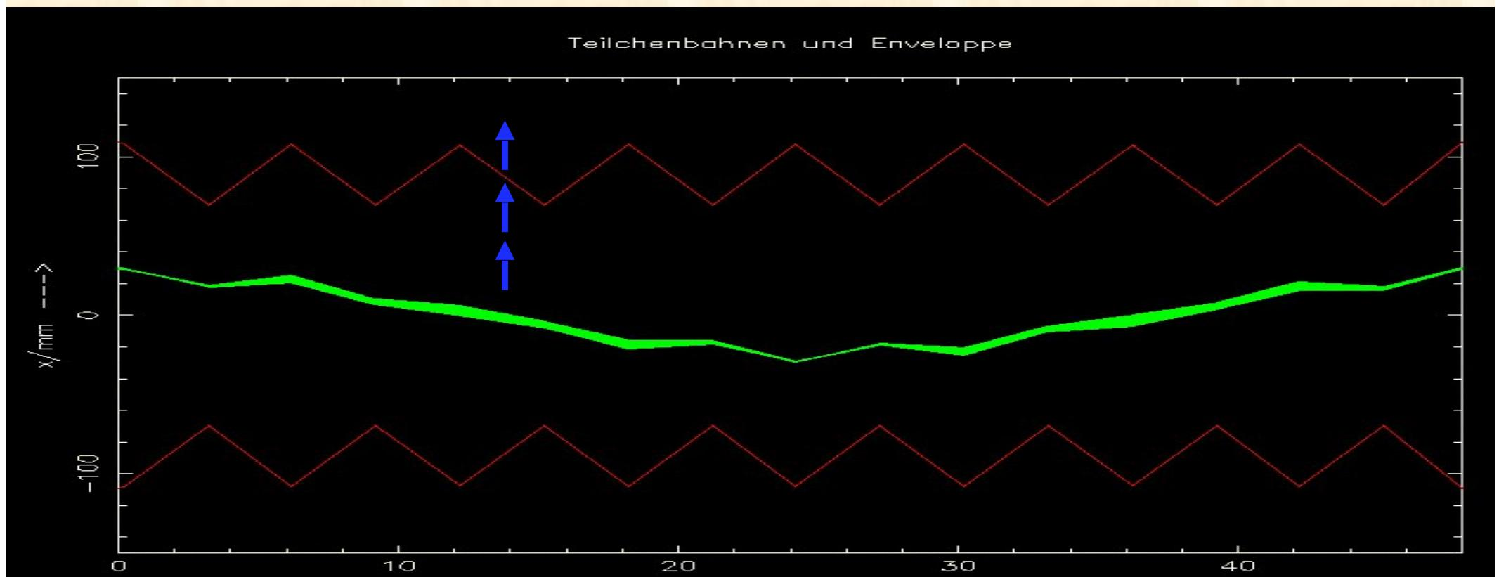
Orbit in case of a small dipole error:
