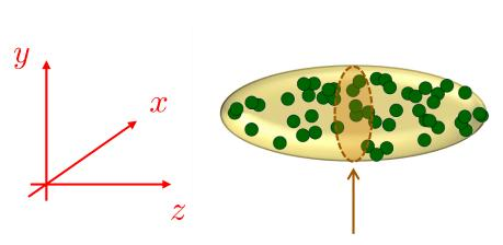
Particles close to the peak line density (often in the bunch center) will have the largest tune spread
