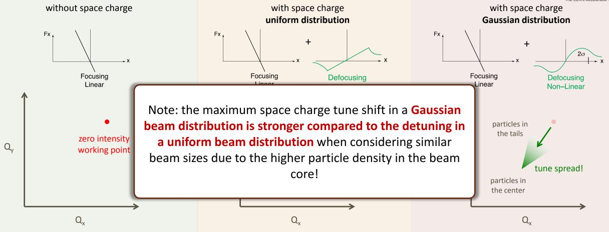
All particles have the tunes Q<sub>x</sub> and Q<sub>y</sub> determined by the machine quadrupoles
