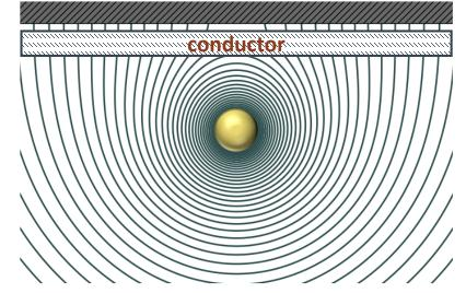
At low frequencies magnetic fields penetrate and pass through the vacuum chamber, they can interact with bodies behind the chamber
