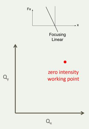
All particles have the tunes Q<sub>x</sub> and Q<sub>y</sub> determined by the machine quadrupoles
