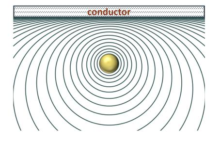
If the skin depth is very small (rapidly varying fields), magnetic fields do not penetrate and the field lines are tangent to the surface.
