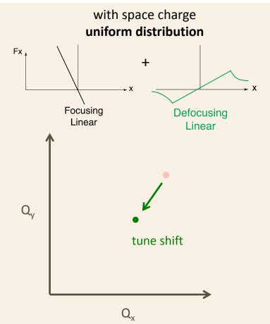
All particles have the tunes Q<sub>x</sub> and Q<sub>y</sub> determined by the machine quadrupoles and the linear defocusing from space charge
