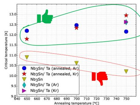
Critical temperature measurement: double coil inductive method [3]
