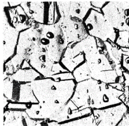
FIG. 1 Step Structure (500×) (Steps between grains, no ditches at grain boundaries)
