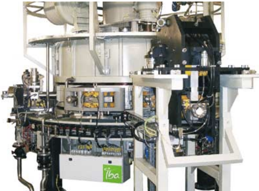
The IBA rhodotron – a commercial accelerator used for e-beam sterilisation
