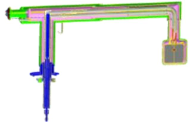
decoupled moderator: solid CH<sub>4</sub> @ 45 K
