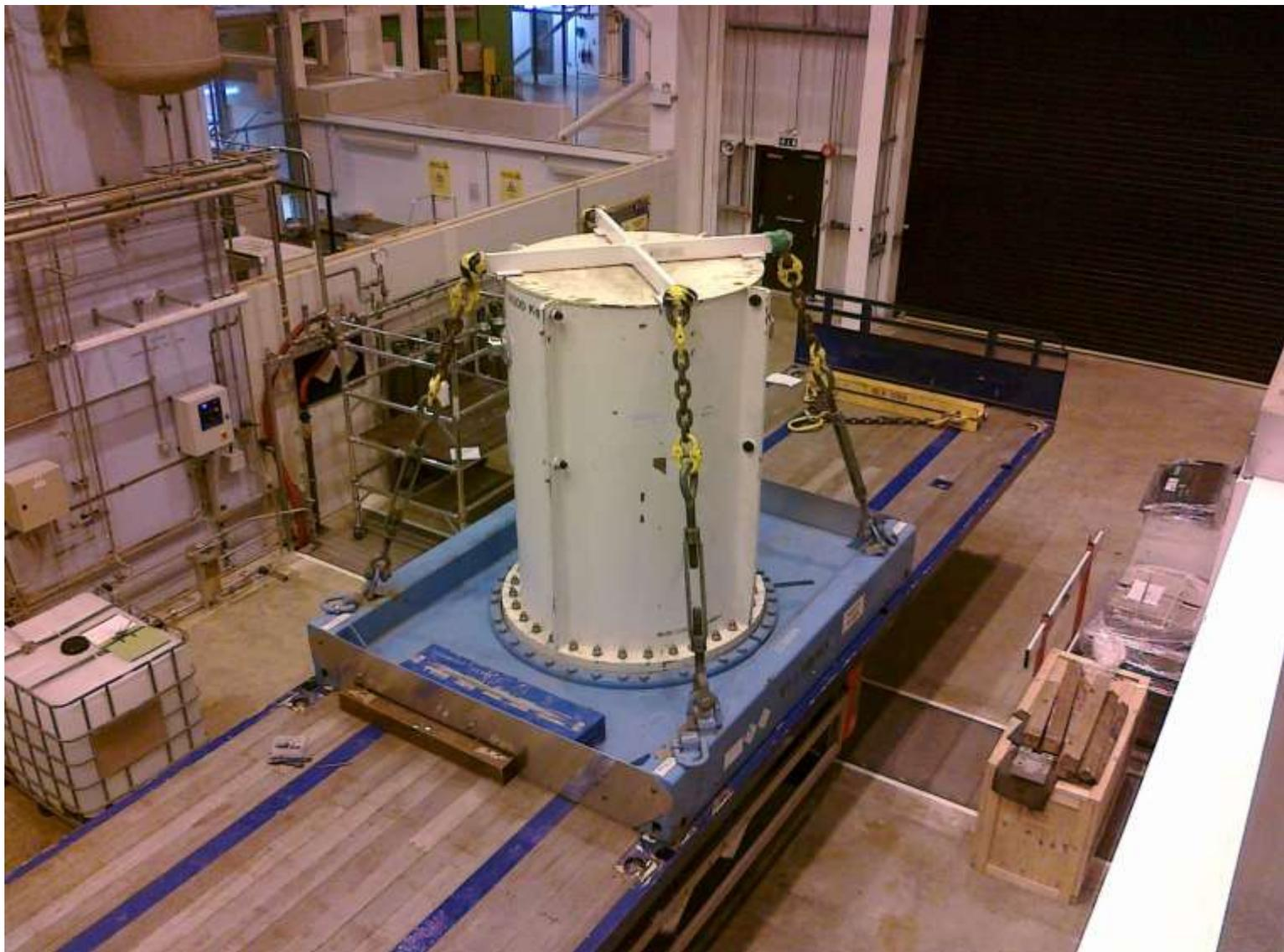
For final disposal the target is transferred to a registered and licenced Type B package and transported to Sellafield the UK's nuclear waste storage facility
