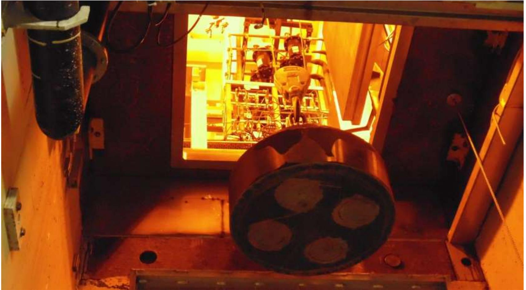
Shield plug is lowered onto flask.
