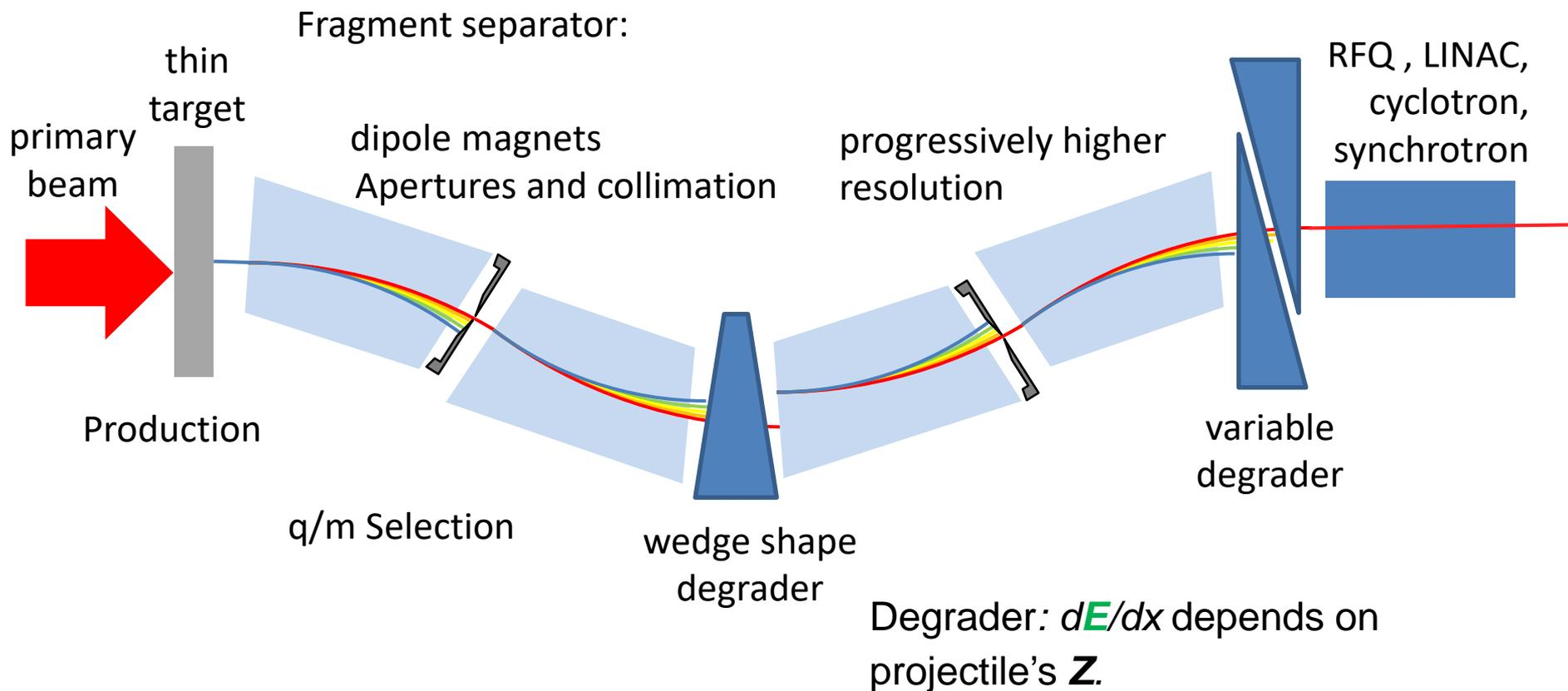
In flight fragmentation suitable for very short half life beams
