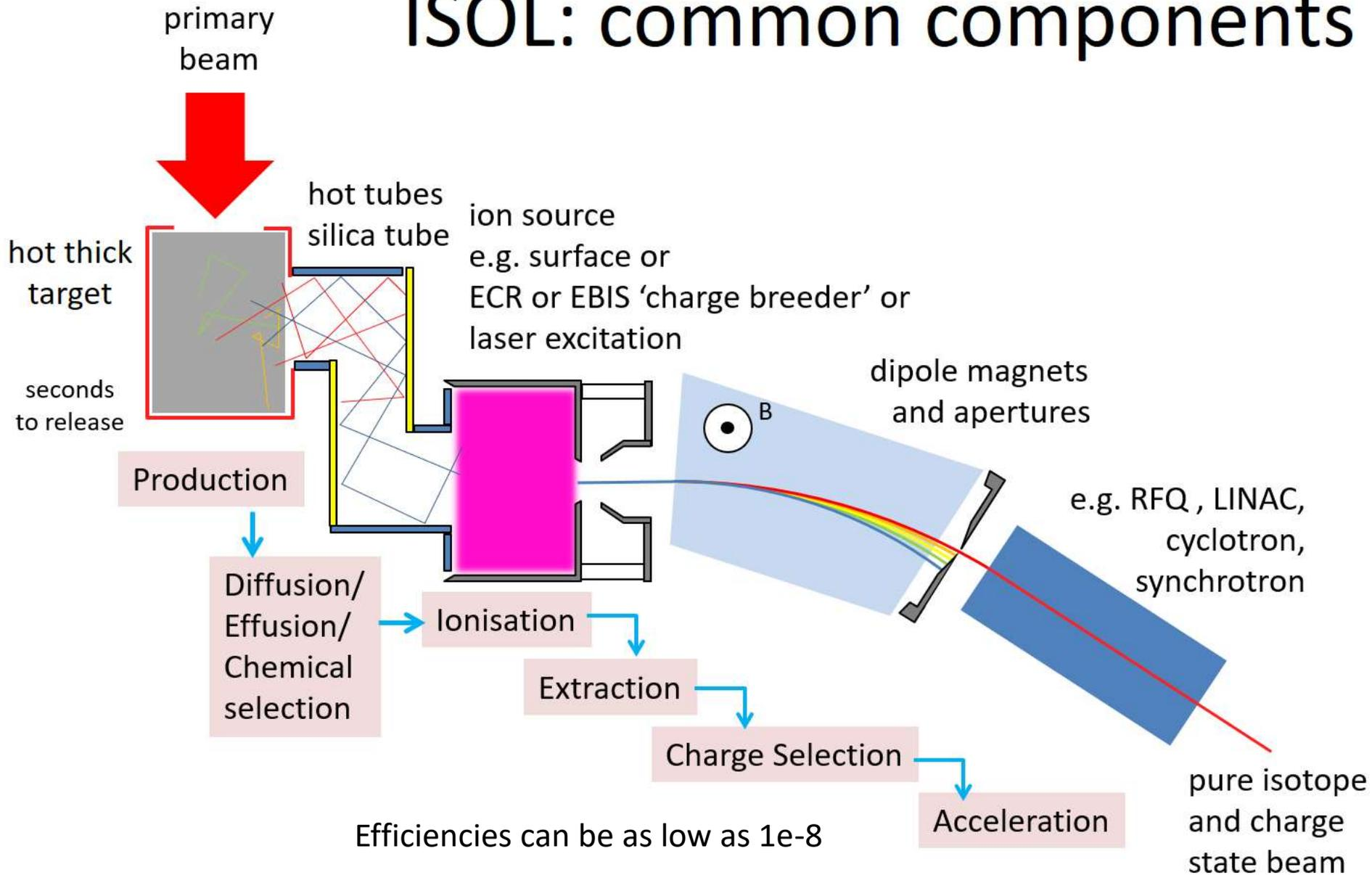
ISOL produces very pure beams with “long” half life
