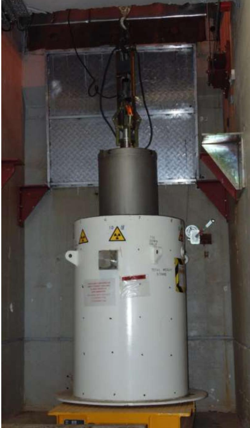
Target and can being lowered into the transport flask
