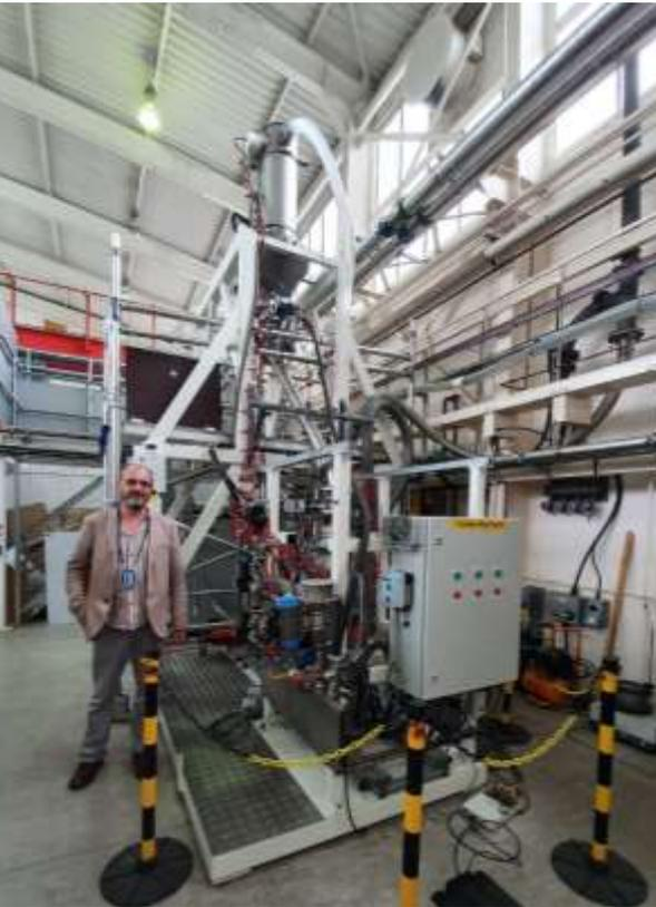
Tungsten powder handling system developed at RAL
