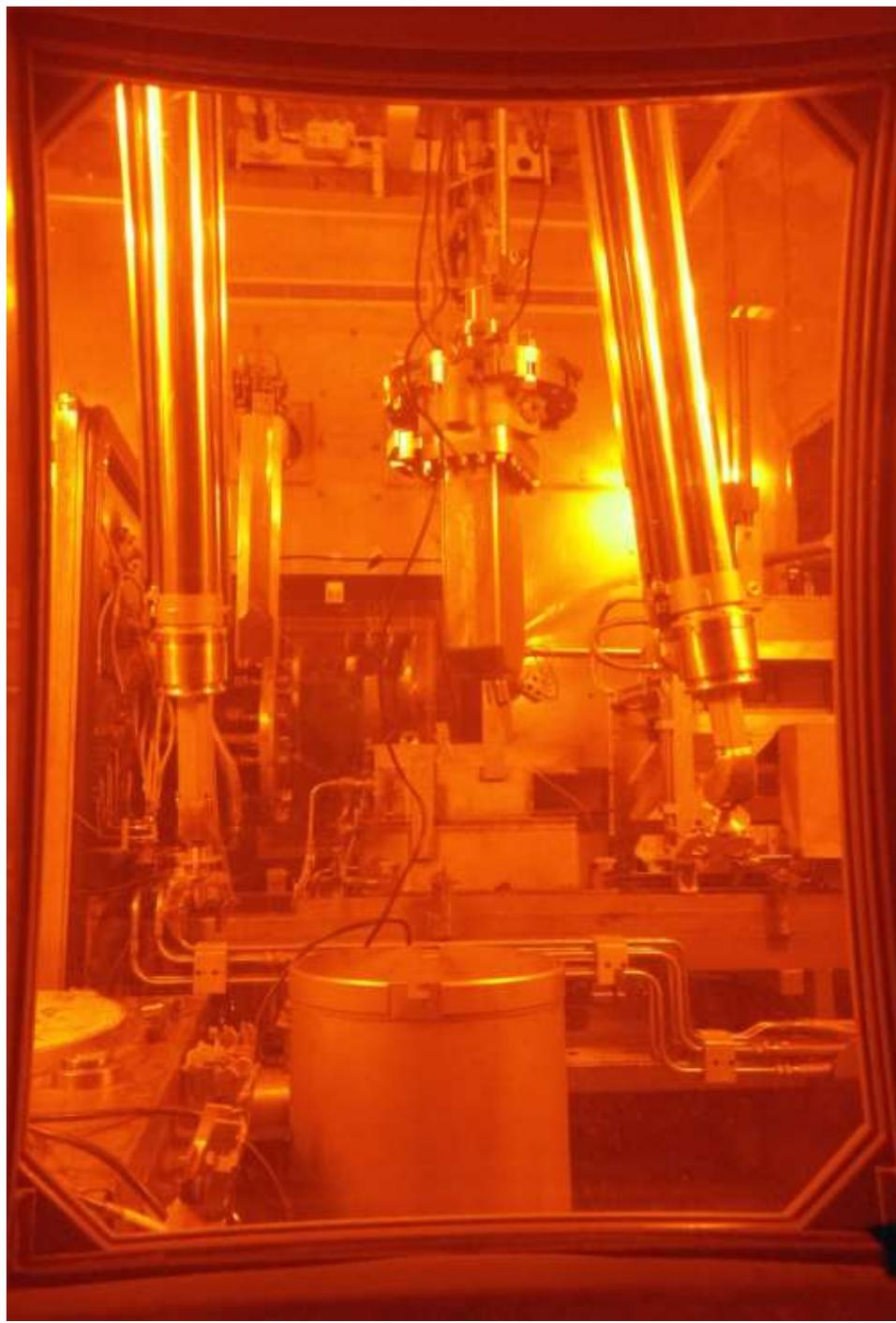
The target being lifted over to the disposal can on the south side of the RHC
