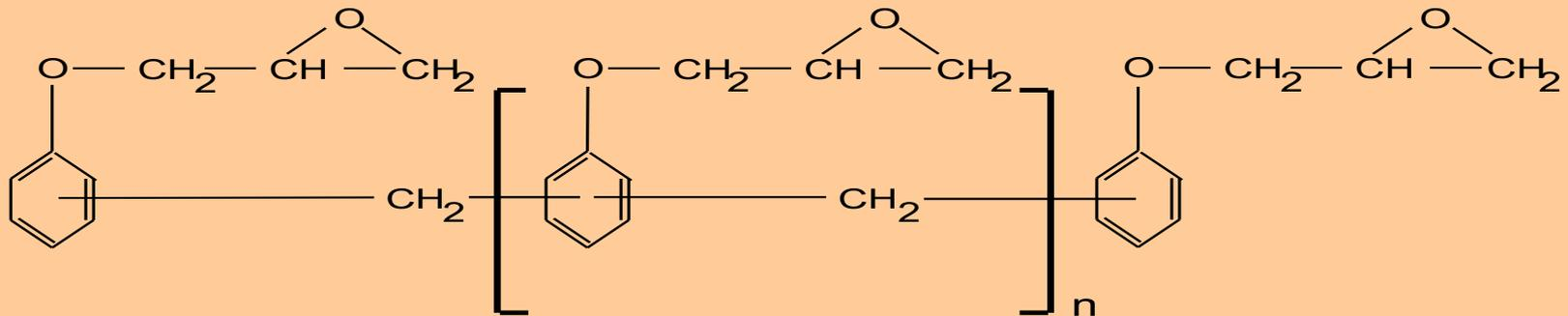
Commercial EPN Resin ( $n = 0.4$  avg) when  $n = 0$ , Resin is (pure) DGEBF
