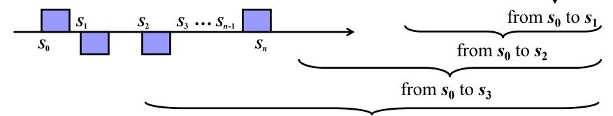
For **periodic beamlines** (i.e. a beamline constructed from a repeated unit), transfer matrix for single period can be parameterised in terms of the **Courant–Snyder parameters**  $(\alpha, \beta, \gamma)$  and the **phase advance**  $\mu$ :
