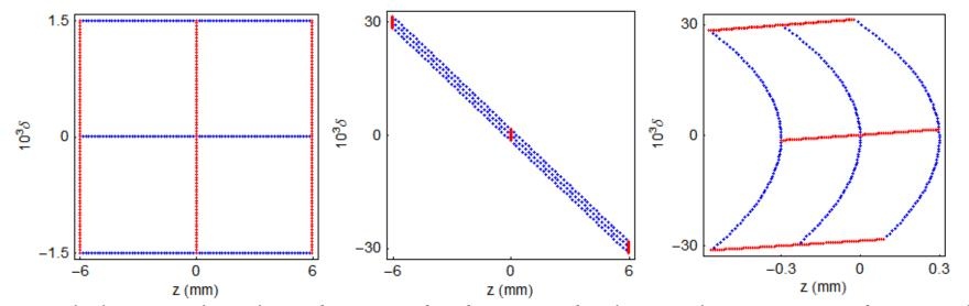
Although the **bunch length** has been **reduced**, there is significant **distortion** of the distribution: the **rms bunch length** will be **significantly longer** than we are aiming for.
