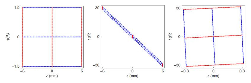
The rms **bunch length** is **reduced** by a factor of 20 as required, but the **rms energy spread** is **increased** by the same factor, because the transfer map is **symplectic**, so phase space areas are conserved under the transformation
