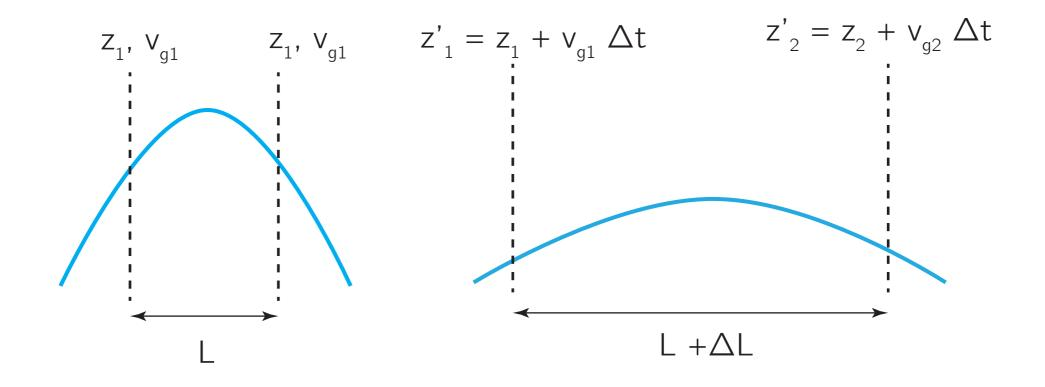
•Longitudinal variation in group velocity changes shape of pulse envelope as it propagates
