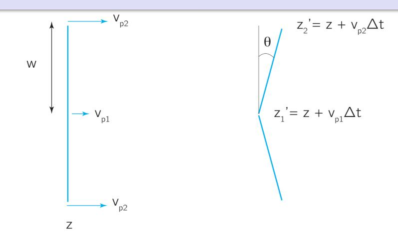
• Transverse gradient of refractive index leads to tilting of wavefront
