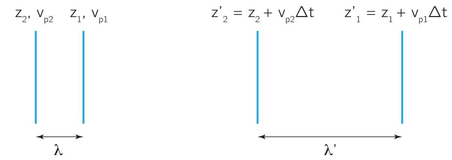
• longitudinal variation in refractive index also means phase velocity varies, leading to a change in the wavelength
