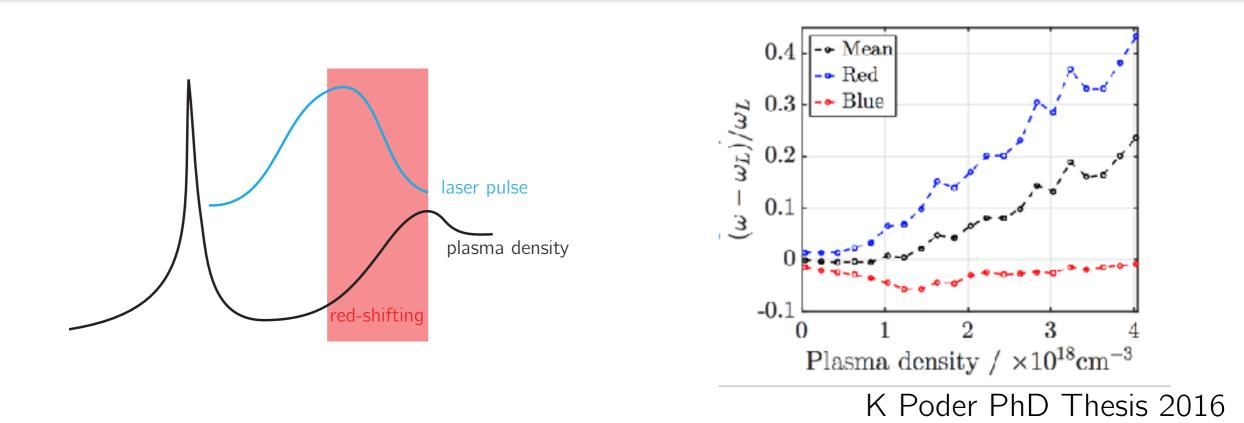
• Refractive index at front of bubble causes red-shifting of photons
