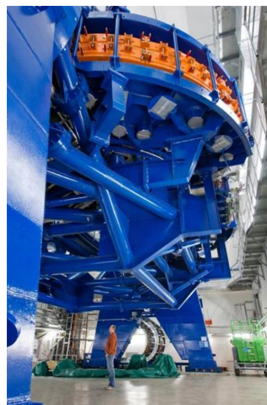
NIRS, superconducting rotating Gantry, 600 tonnes, Heidelberg, operating since November 2012.
