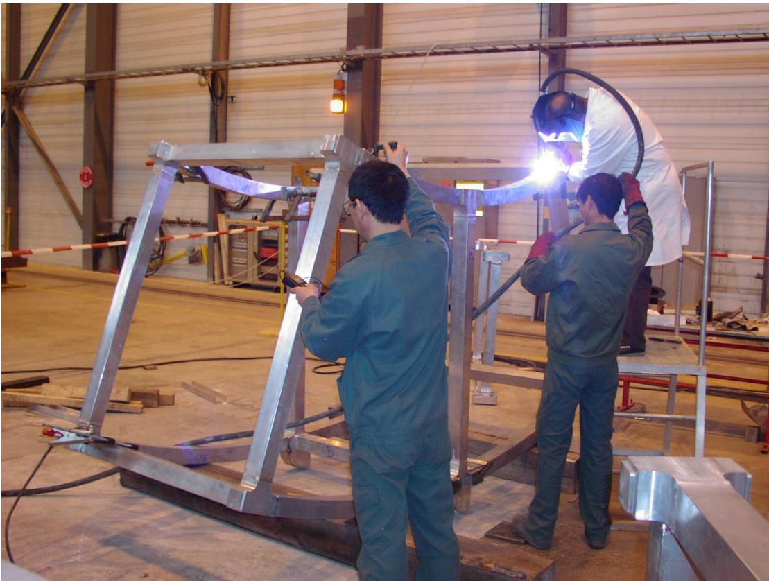
Use of inserts to avoid welds in the stress concentration zone. AW 6082 T4
