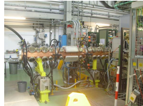
The CERN Linac4 RFQ 45 keV – 3 MeV, 3 m 80 mA H-, max. 10% duty cycle
