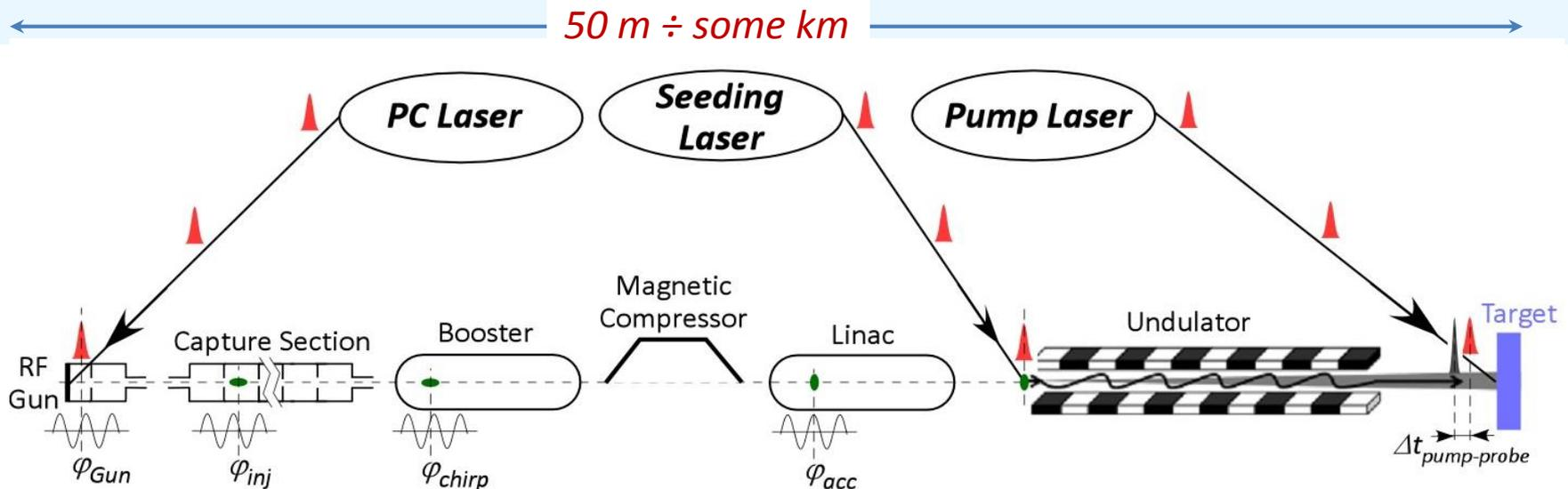
Naive approach: can each sub-system be synchronized to a local high-stability clock to have a good global synchronization of the whole facility ?
