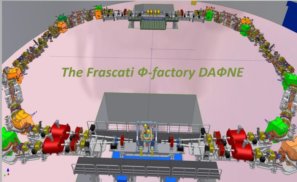
Bunches of the 2 colliding beams need to **arrive** at the **Interaction Point** (max vertical focalization) at the same time.
