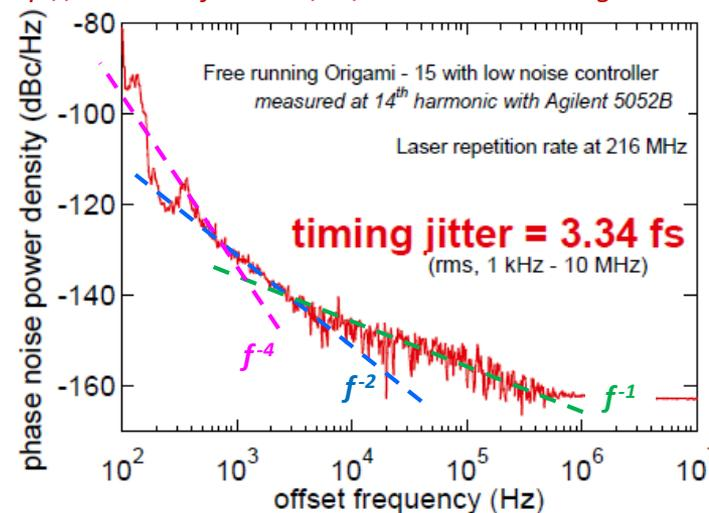
OMO – Mode-locked laser –  $f = 3024$  MHz
