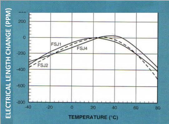
Around some optimal temperature  $T_{opt}$  cable physical elongation is compensated by dielectric constant variation. PPM relative delay variation is:
