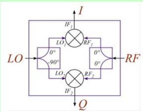
$$\begin{cases} V_I = k_{CL} A_{RF} \cos(\varphi) + \text{high harmonics} \\ V_Q = k_{CL} A_{RF} \sin(\varphi) + \text{high harmonics} \end{cases} \Rightarrow \begin{cases} A_{RF} \div \sqrt{V_I^2 + V_Q^2} \\ \varphi = \arctan(V_Q/V_I) + \frac{\pi}{2} [1 - \text{sgn}(V_I)] \end{cases}$$
