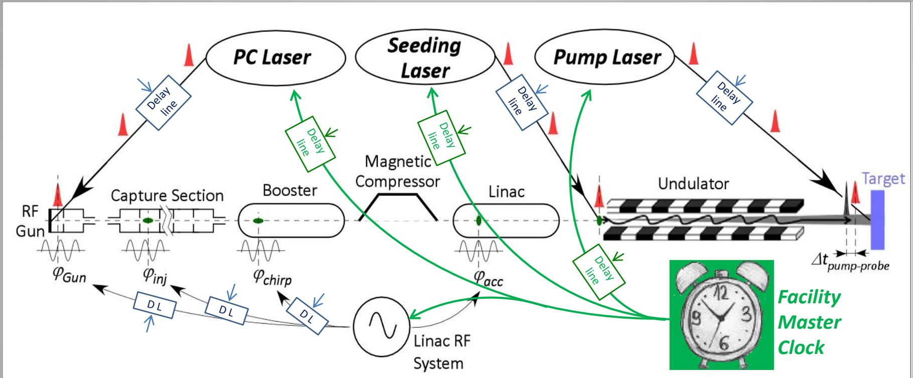
Once the local oscillators have been locked to the reference, they can be shifted in time by means of delay lines of various types – translation stages with mirrors for lasers, trombone-lines or electrical phase shifters for RF signals. This allows setting, correcting, optimizing and changing the working point of the facility synchronization.
