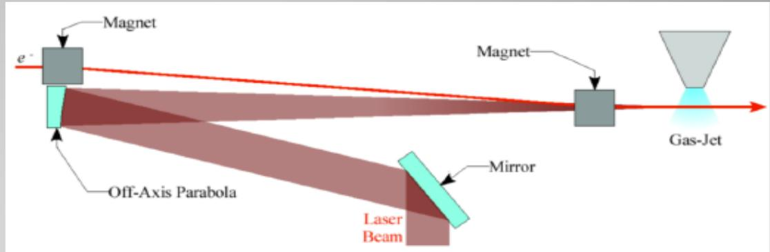
To produce good quality beams external bunches have to be injected in the plasma wave. The “accelerating buckets” in the plasma wave are typically few 100  $\mu\text{m}$  long.
