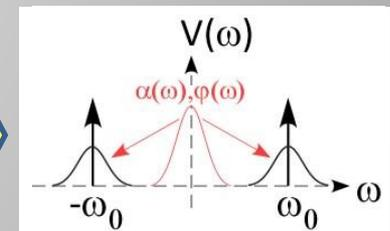
In real oscillators the amplitude and phase will always fluctuate in time by a certain amount because of the unavoidable presence of noise. However, by common sense, a well behaving real oscillator has to satisfy the following conditions:
