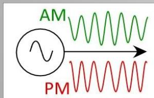
$$V(t) = V_0 \cdot [1 + \alpha(t)] \cdot \cos[\omega_0 t + \varphi(t)]$$
