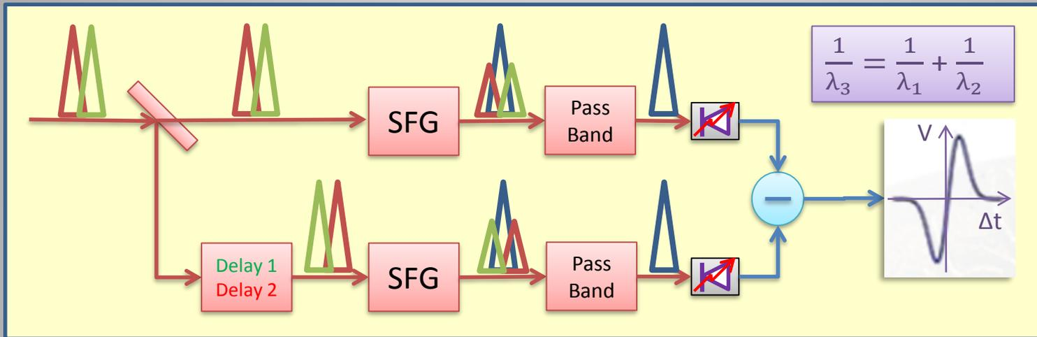
The two pulses have orthogonal polarization and generate a shorter wavelength pulse proportional to their time overlap in each branch by means of non-linear crystal.
