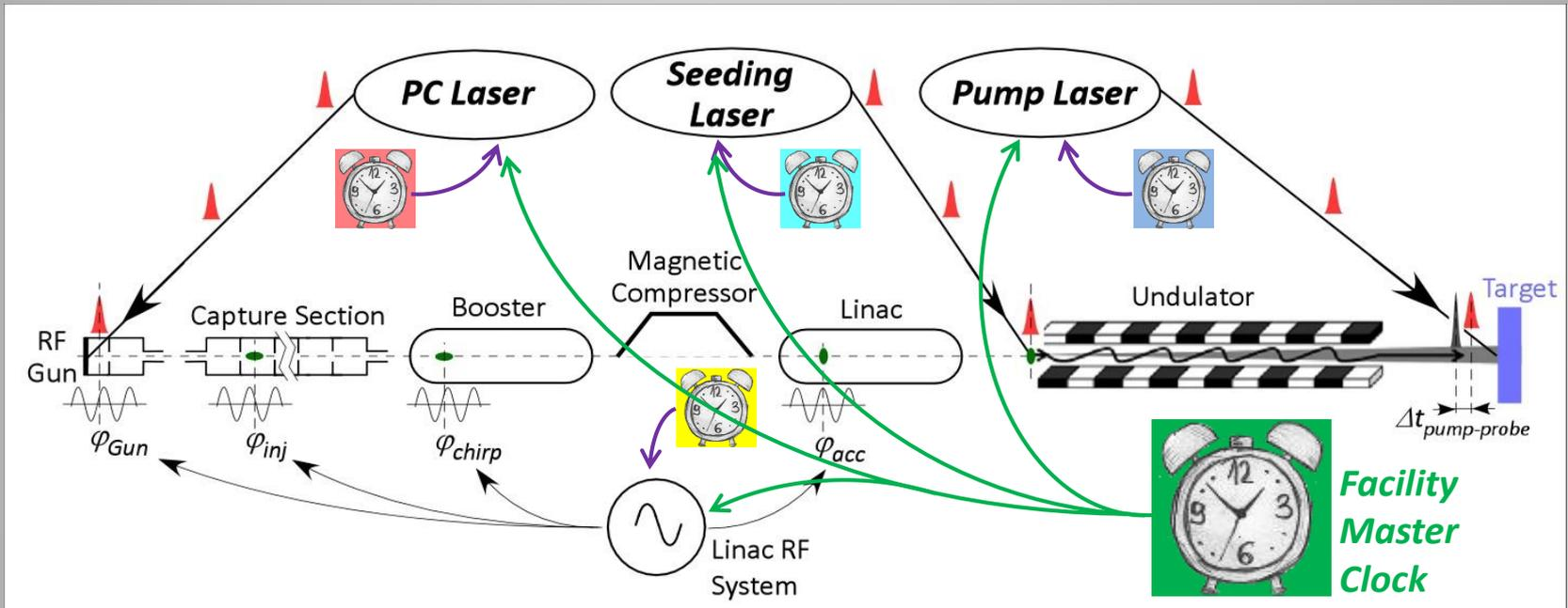
**Best optical clocks**  $\rightarrow \Delta\omega/\omega \approx 10^{-18} \rightarrow \Delta T/T \approx 10^{-18} \rightarrow T \approx 10 \text{ fs}/10^{-18} \approx \underline{\underline{3 \text{ hours !!!}}}$
