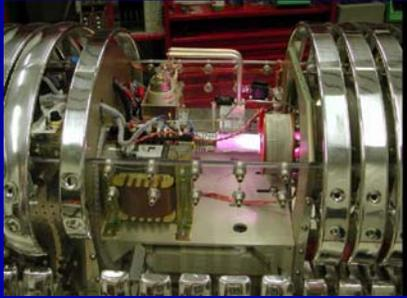
400 kV electrostatic accelerator (High Voltage Engineering Europe):
