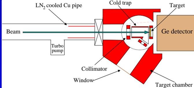
The experimental strategy consists in setting the beam energy at 1 keV above the resonance energy and varying it in steps of 10 eV with a positive voltage applied to the thick target of <sup>25</sup>Mg.
