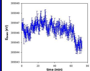
The long term stability of the accelerator is monitored with the yield variation observed setting the proton beam energy exactly at the resonance value.
