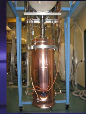
RF tests were performed at TRIUMF SCRF lab in Vancouver, Canada. During the rinsing a small fraction of a ring shape of the Nb coating peeled off in the high electric field region. It was anyway decided to proceed with the RF test.
