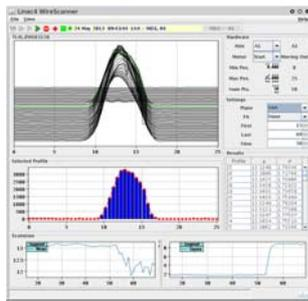
Transverse profile acquired by using the emittance meter slit as a scanning scraper and by measuring the transmission with a downstream current transformer
