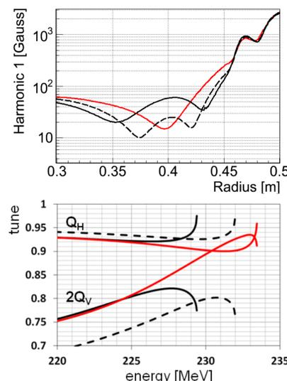
Figure 3: (top) First harmonic component and (bottom) tune functions: red full line= measured with a slightly horizontally displaced main coil, black full line= measured with a horizontally centered main coil, black dashed line= from the calculated OPERA3D field map.
