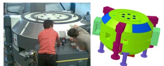
Figure 6: (left) shims applied on the S2C2 (may 2013) (right) OPERA3D model of the S2C2 with all shims included on the top yoke.
