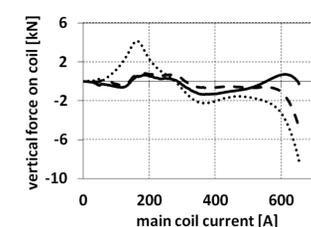
Figure 5: Measured total vertical force on the main coil. Dotted line= during the initial ramp-up, dashed line= after vertical positioning of the main coil and full line= after application of all shims on the top yoke.
