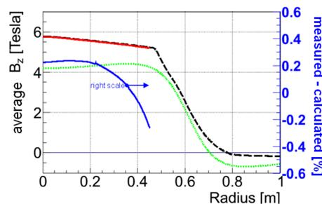
Figure 2: Average field in the S2C2. Red full line= measured, black dashed line= calculated with OPERA3D, green dotted line= calculated pure coil field, blue full line (right scale)= deviation between measured and calculated average field.
