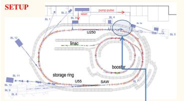
Sketch of the DELTA facility: DELTA is a synchrotron light source with a beam energy of 1.5 GeV, a beam current up to 130 mA in multibunch mode, and a revolution frequency of 2.6 MHz.
