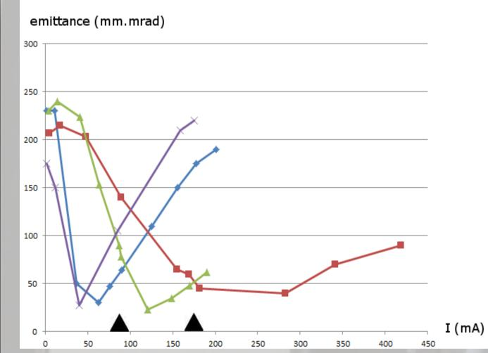
The halfenergy/halfintensity beam has about the same beahvior with a \u03c612mm aperture, the \u03c68mm results have to be compared with the loss levels at some intensities, affecting the emitance.
