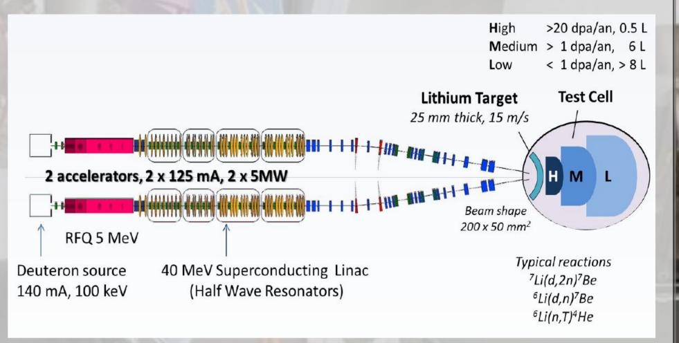
A continuous beam of 2x125mA medium energy (40MeV) Deuteron ions is sent on the liquid Lithium target for a total of 10MW. The flux of generated neutrons will then irradiate the test cells.
