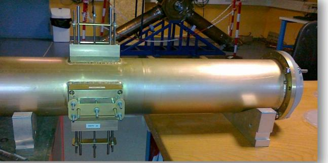
CoStub replaces the coaxial between CaCo and the IOT's and allows to short-circuit the waveguide when working only with one IOT.
