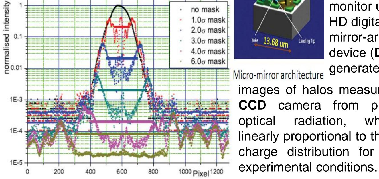
The DMD masking technique generates a reflective mask *i.e.* to reject the intense light from the core with very high efficiency at a large angle away from the optical path before reaching the camera optics. Normalized scans of He-Ne laser images with various mask sizes shows how effective the DMD masking method is in profile thresholding.
