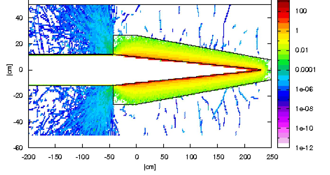
• Cone made from Cu (length: 2.94 m, max. ø: 0.265 m) • Beam characteristics: two dimensional Gaussian distribution, radius: 2.5 cm, divergence: 150 mrad
