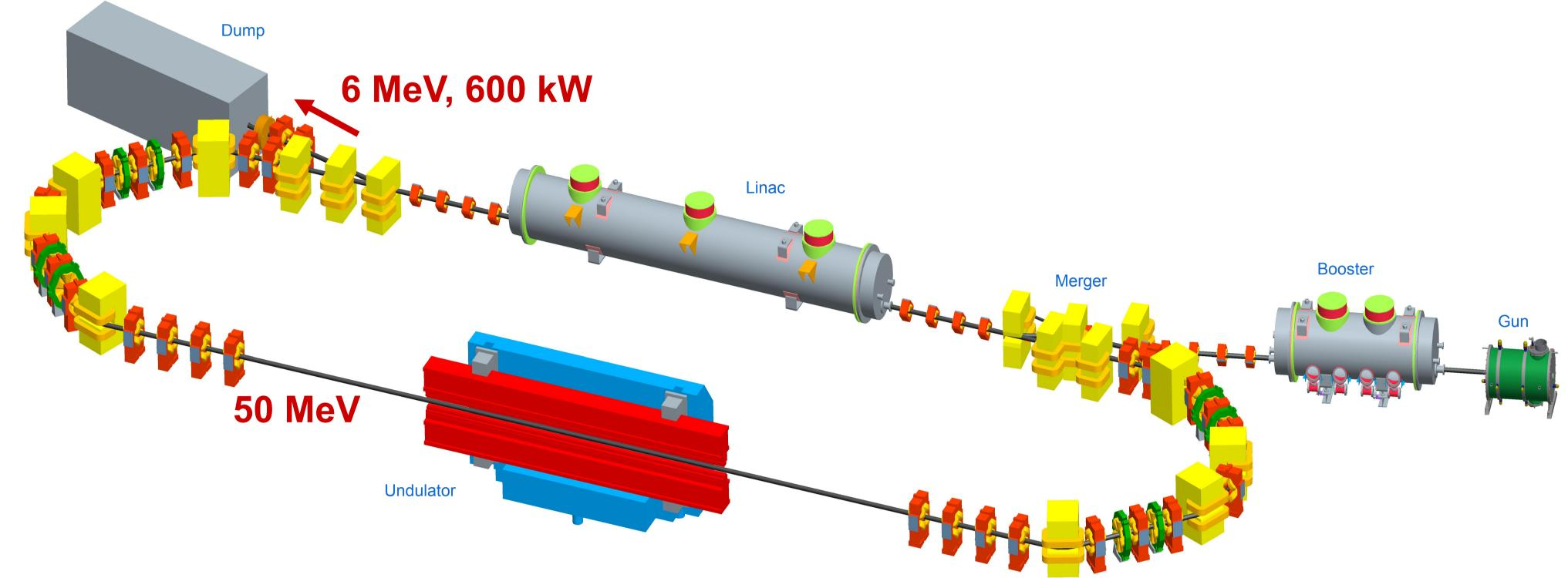
Challenge: Low penetration depth at 6 MeV, but high power leads to heating of the beam dump surface.
