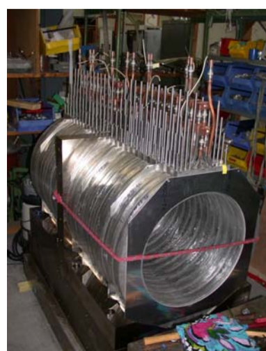
Assembly of a radiation hard solenoid magnet
