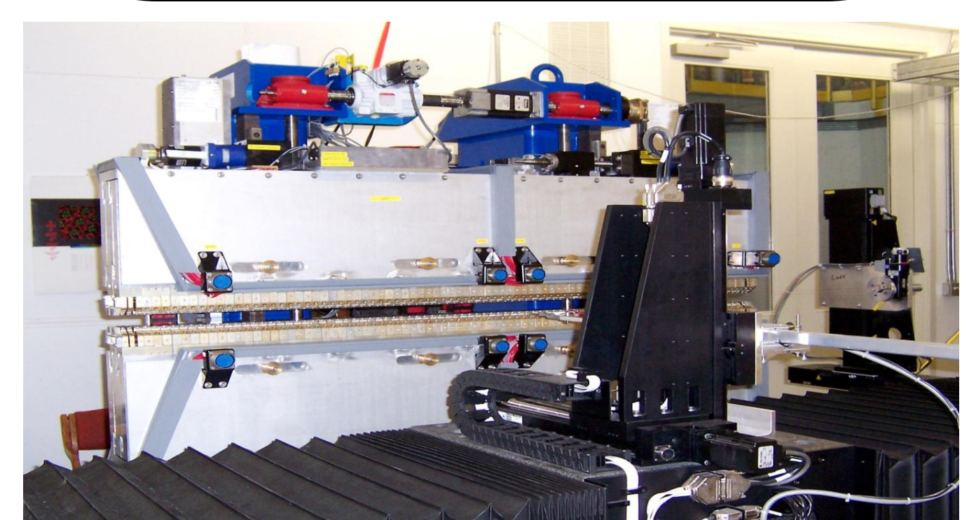
SM EPU including mounted correction coils, multipole trim magnets, and Hall probe bench (front)
