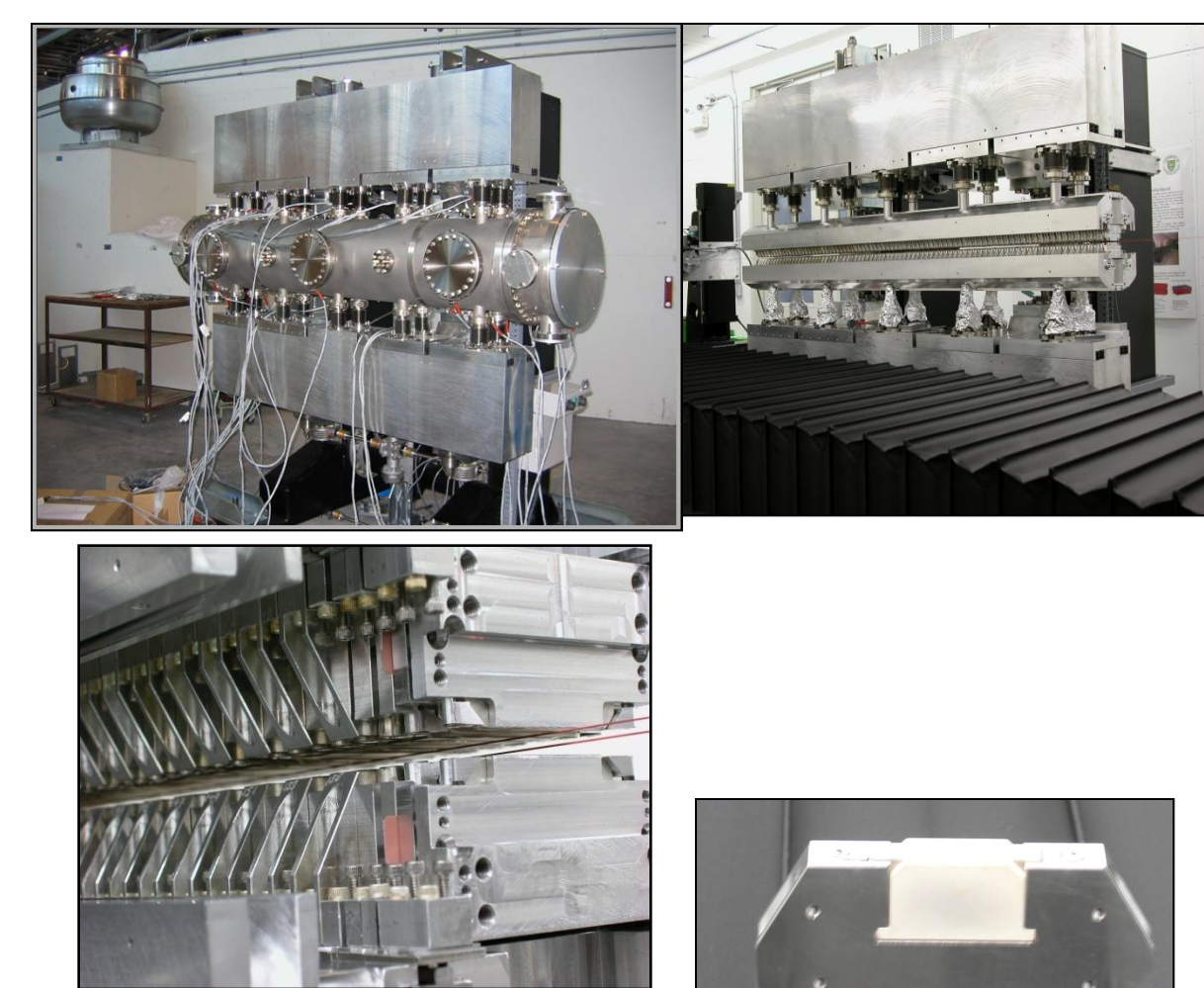
SGU support structure, vacuum chamber magnetic assembly, single pole piece
