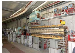
The IR-Undulator in the FLASH tunnel
