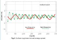
It has been shown that in what concerns the wall resistivity, it is preferable to have a rectangular or elliptic cross-section vacuum chamber with Aluminium made walls knowing the fact that its a shorter relaxation time (in AC electrical conductivity) makes the wakes ring less. As for the surface induced wakes, calculations indicate that the induced energy spread would account for about 12 % and 15 % of the resistivity induced energy spread, respectively for the medium and long FERMI FEL bunch.
