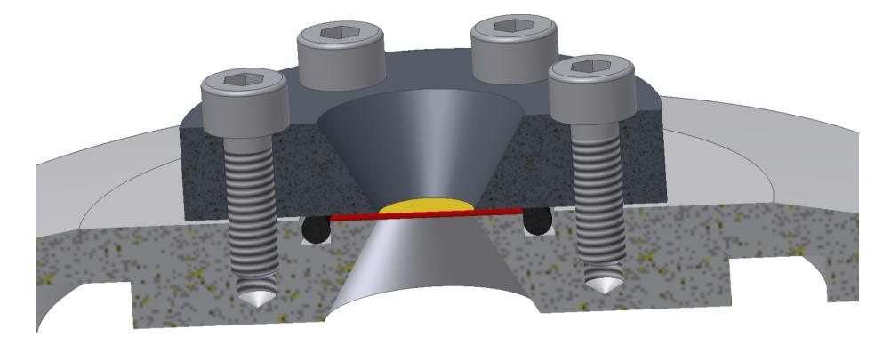
Cross-section schematic of exit flange (Ø 4cm): sealing O-ring (black), extraction foil (yellow) and optional mesh for support (red). Aperture size is 5 mm.
