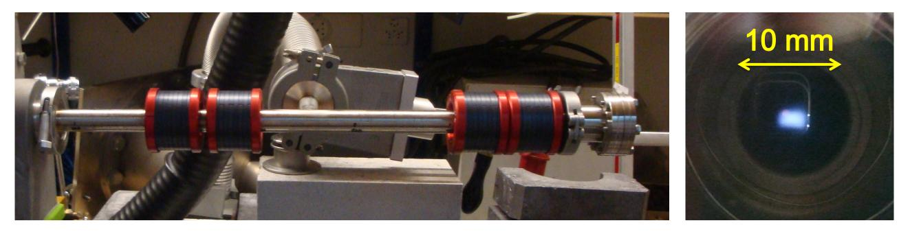
• Left: HEBT (length 55cm) consisting of four permanent magnet quadrupoles *Right: focussed beam made visible on glass scintillator (image size 2x2 cm<sup>2</sup>)*
