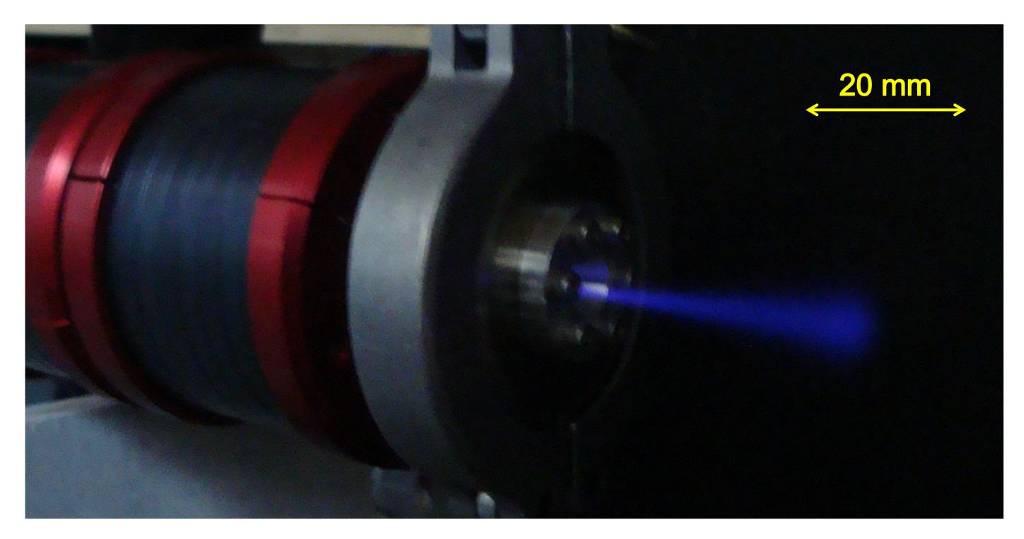
Beam extraction system: a vacuum-tight exit flange containing a 5 µm steel foil marks the end of the 2 MeV beam line. The H<sup>-</sup> ions pass through the foil, thereby being stripped of electrons and losing approx. 0.5 MeV kinetic energy. The extracted proton beam is visible by eye (blue glow) through excitation of the air. The beam continues depositing energy and starts to grow, the widest and brightest part at the end indicates the Bragg peak.
