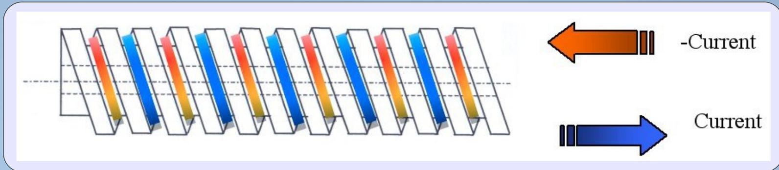
Multi-wire winding model in Opera 3d
