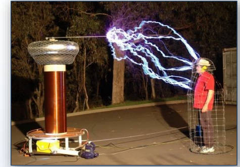
Faraday cage used to protect a person while demonstrating discharges from Tesla transformer
