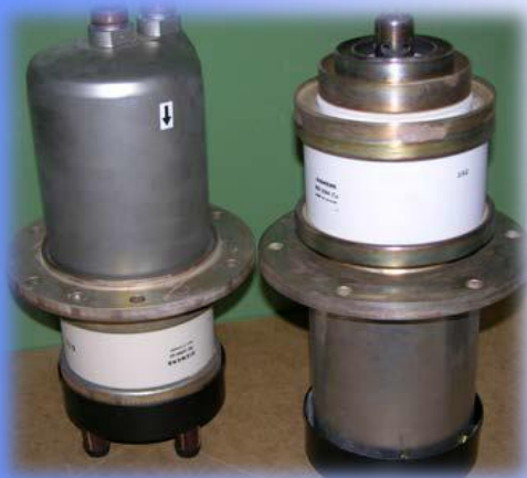
Thales RS 1084 CJ < 30 MHz, 75 kW \eta < 78% (class B)
