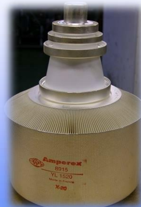
YL1520 (ex Philips, now Richardson), < 260 MHz, 25 kW
