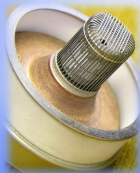
4CX250B (Eimac/CPI), < 500 MHz, 600 W (Anode removed)
