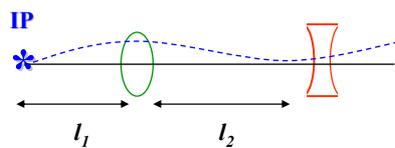
$$\beta(s) = \left(1 + \frac{l_2}{f_1}\right)^2 \beta^* + \frac{1}{\beta^*} \left(l_1 + l_2 + \frac{l_1 l_2}{f_1}\right)^2$$
