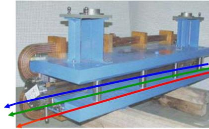
particles with different momentum are running on a different closed orbit
