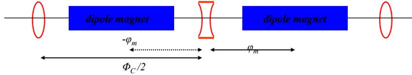
Transformation of  $C(s)$  from the symmetry point in the foc. quad to the center of the dipole:
