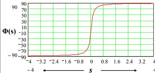
summing the drift spaces on both sides of the IP the **phase advance of a mini β insertion is approximately π**, in other words: **the tune will increase by half an integer.**
