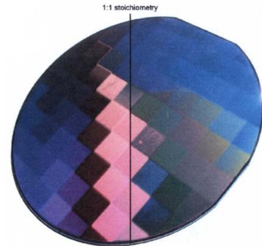
FIGURE 4. Daylight scattered image of a 4-inch Silicon wafer implanted with Cd and Se with the herein discussed parameters and dose d_0 of 2.85 \times 10^{16} \text{ cm}^{-2} .
