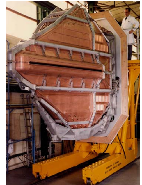
Fig. 26: Outer shell of resonator, with support frame and beam slit
