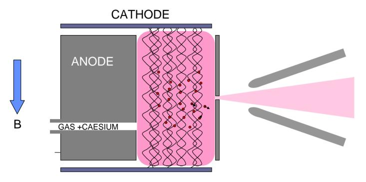
Electrons are extracted along with negative ions! Electron current can be reduced with a dipole B field in extraction.
