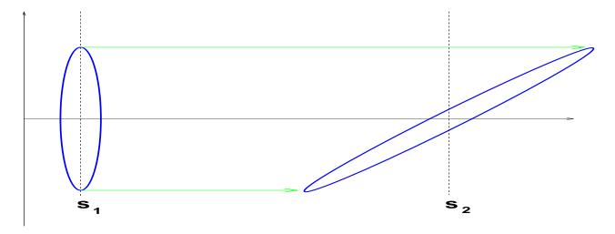
$$\begin{pmatrix} \beta \\ \alpha \\ \gamma \end{pmatrix}_{s_2} = \begin{pmatrix} 1 & -2L & L^2 \\ 0 & 1 & -L \\ 0 & 0 & 1 \end{pmatrix} \circ \begin{pmatrix} \beta \\ \alpha \\ \gamma \end{pmatrix}_{s_1} = \begin{pmatrix} \beta_0 - 2L\alpha_0 + L^2\gamma_0 \\ \alpha_0 - L\gamma_0 \\ \gamma_0 \end{pmatrix}_{s_2}$$
