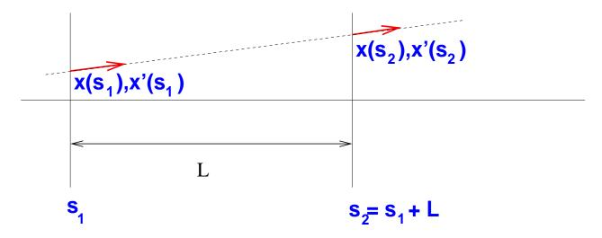
$$\begin{pmatrix} x \\ x' \end{pmatrix}_{s_2} = \begin{pmatrix} x \\ x' \end{pmatrix}_{s_1} + \begin{pmatrix} x' \cdot L \\ 0 \end{pmatrix}_{s_1} = \begin{pmatrix} 1 & L \\ 0 & 1 \end{pmatrix} \circ \begin{pmatrix} x \\ x' \end{pmatrix}_{s_1}$$
