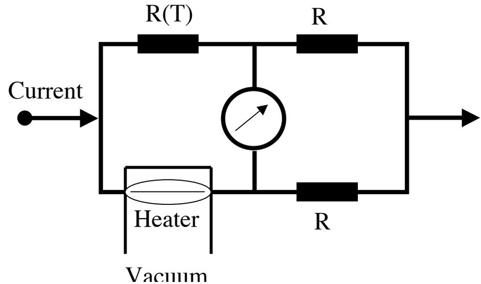
A resistor with a large temperature coefficient is mounted inside the vacuum and is heated to a constant temperature. The required heating current to maintain the bridge balanced is a measure of the pressure.
