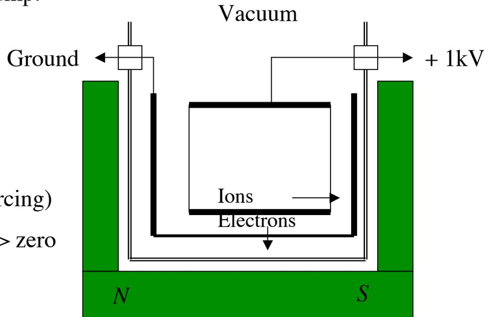
Leakage current in the cables and in the gauge can simulate a higher pressure.
