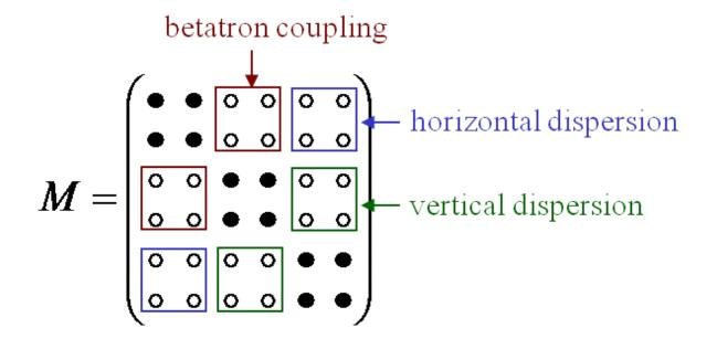
The formula we derived for the natural emittance assumed no betatron coupling, and that the coupling between the horizontal and longitudinal motion was relatively weak.
