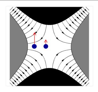
In a storage ring, skew quadrupole fields ofen arise from quadrupole tilts, and from vertical alignment errors on sextupoles.
