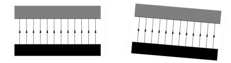
vertical misalignment of a quadrupole, so that there is a horizontal magnetic field at the location of the reference trajectory:
