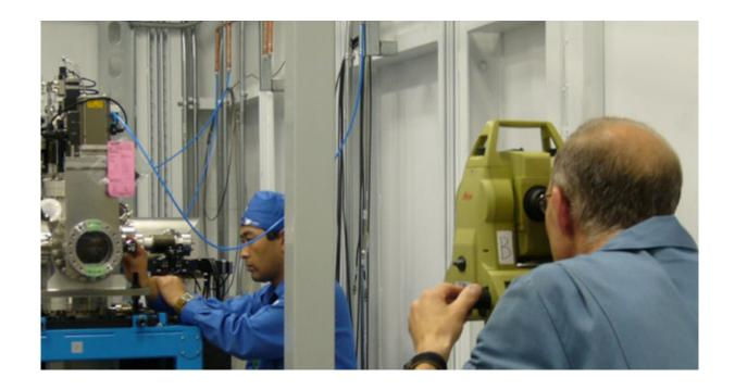
Step 2: Determine the positions of the BPMs relative to the quadrupoles.
