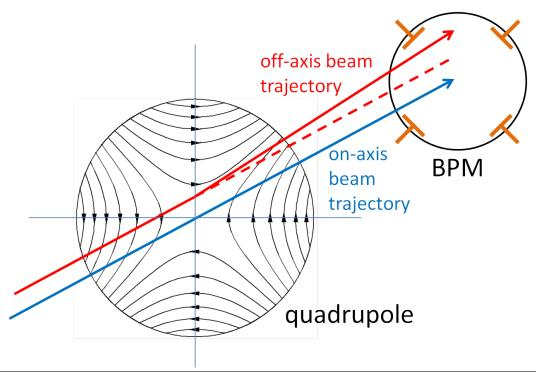
Step 3: Correct the orbit (using steering magnets) so that it is as close as possible to the centres of the quadrupoles.
