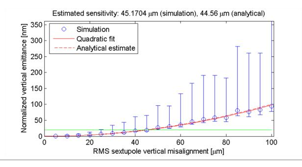
The formulae we have derived so far are useful for developing a "feel" for how the vertical emittance depends on magnet alignment errors, and for making rough estimates of the sensitivity to particular types of error.
