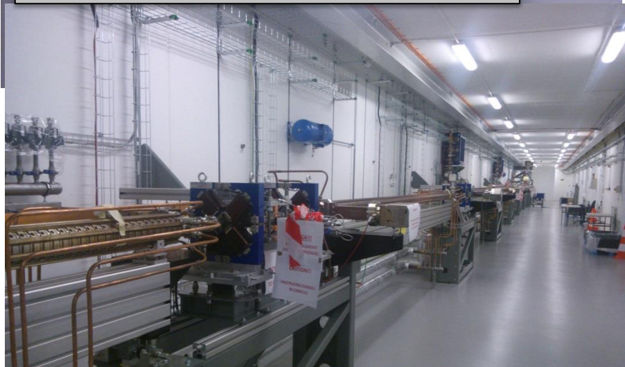
Linac and waveguide system up to the transfer line and installed under vacuum
