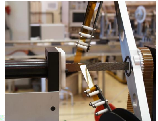
Cable insulation by double polyimide wrap
