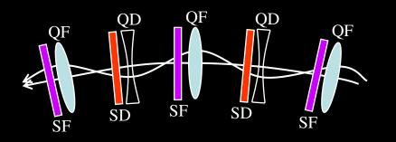
Characteristic Frequency of the Magnetic Lattice Given by the strength of the Quadrupole magnets
