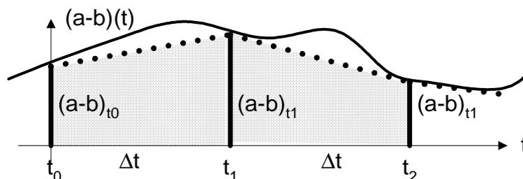
Besides the two shown fixed step solver ( $\Delta t = \text{constant}$ ), solvers exist, which adapt the time step to the function that has to be integrated. They are very useful for systems that contain switching actions.
