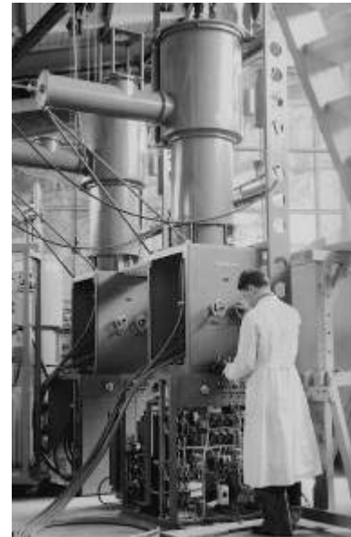
200 MHz triode amplifier (CERN Linac3)
