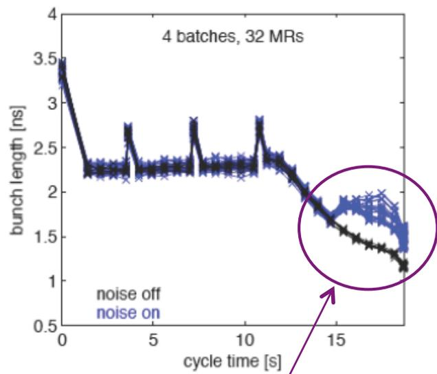
*In the last part of the SPS cycle for LHC beams, the longitudinal emittance is blown up for beam stability (4<sup>th</sup> harmonic cavity)*
