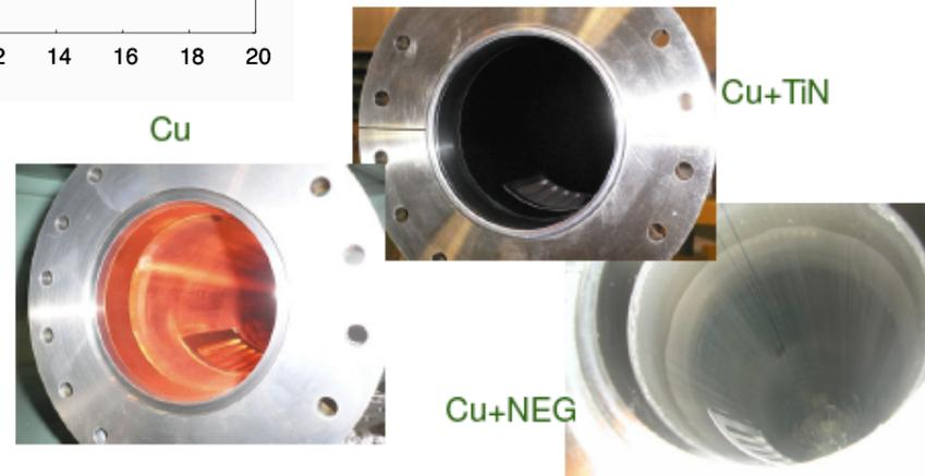
Different coatings and grooved surfaces applied in KEK-B
