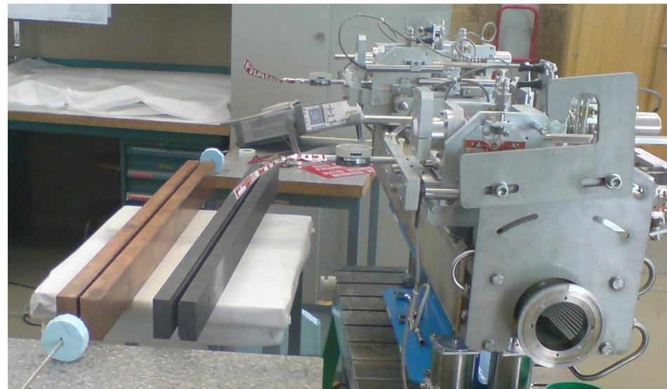
LHC collimator prototypes in copper and graphite
