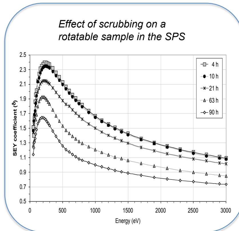
Measured SEYs and electron clouds for amorphous Carbon coatings
