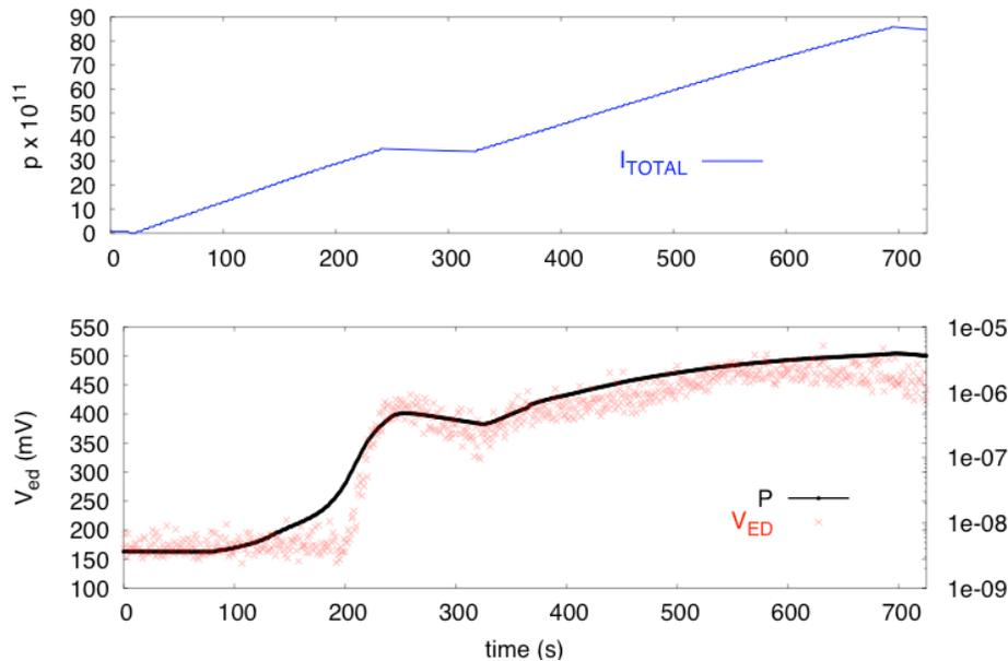
*Pressure rise observed in RHIC when the number of injected protons reached  $30e11$ , with correlated  $e$ -cloud signal*
