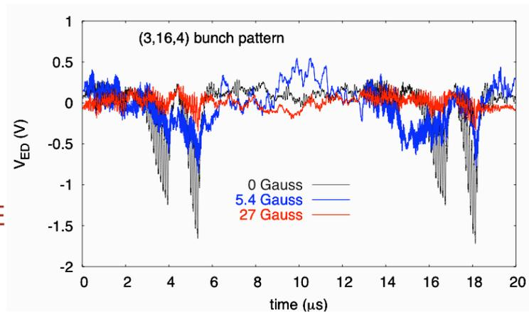
← Effect of a solenoid in RHIC
