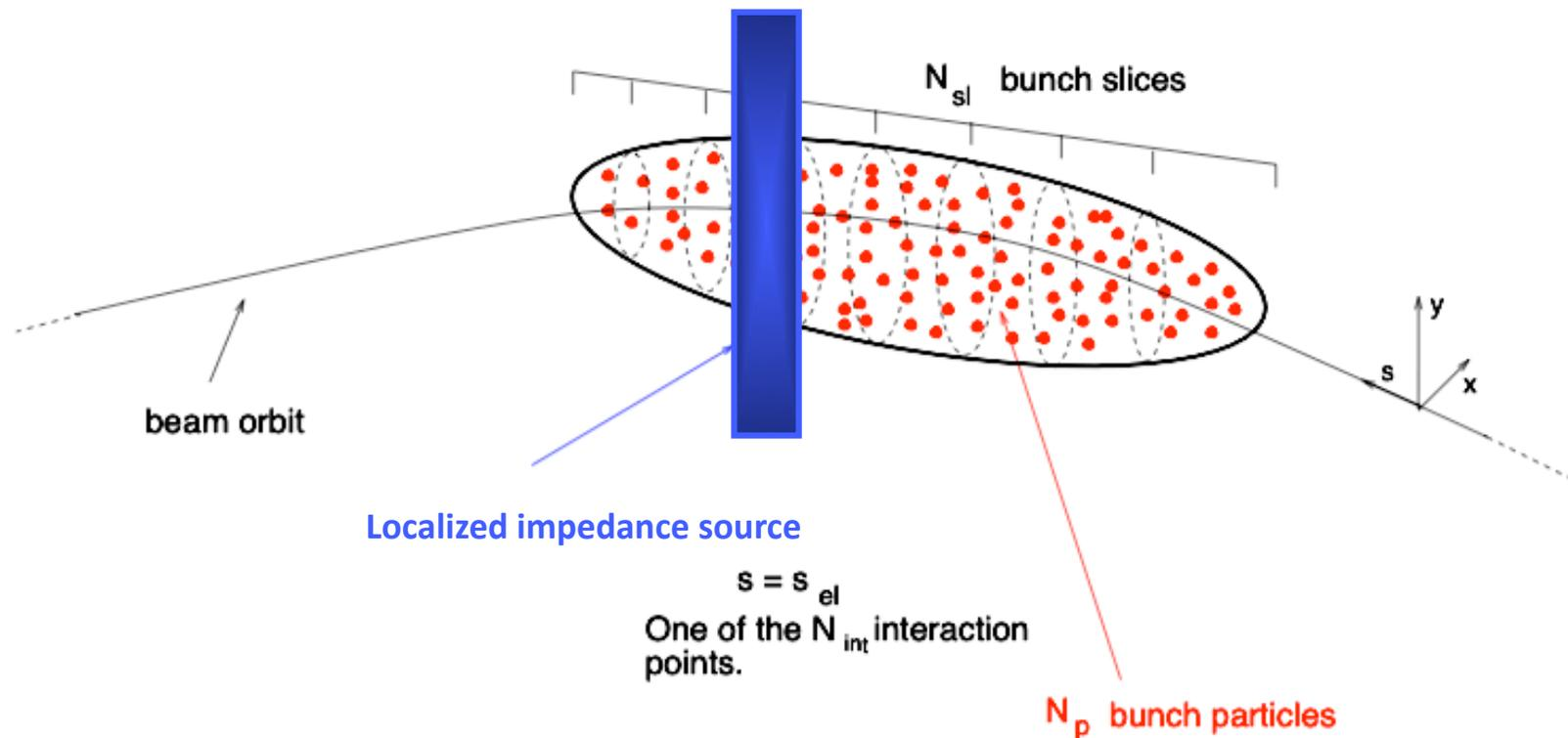
The collective interaction is lumped in one or more points along the ring (**kick points**), where the subsequent slices of a bunch (macroparticles) interact with an impedance (through the wake) or with an electron cloud
