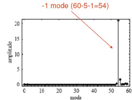
*The electron cloud single-bunch instability at the SPS. Only the last few bunches of the 4th train injected are lost after reducing the vertical chromaticity!*
