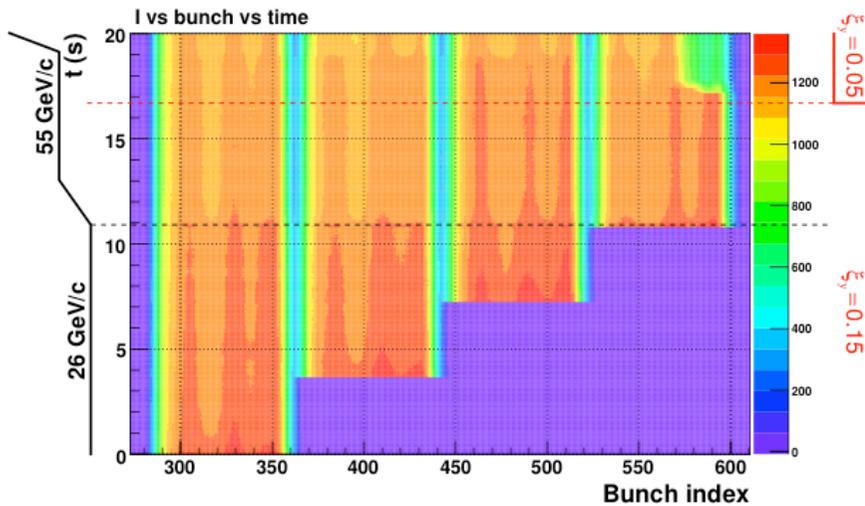
*An example of horizontal coupled bunch instability driven by electron cloud at DAFNE in Frascati*
