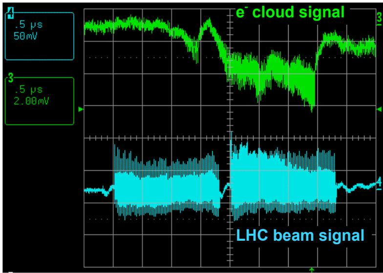
Signal from a pick-up with two bunch trains (LHC-type) inside the SPS
