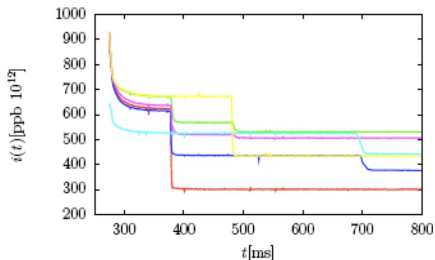
*Depending on the injected intensity, the PS-Booster can lose the beam at several points along the cycle when the transverse feedback is switched off*
