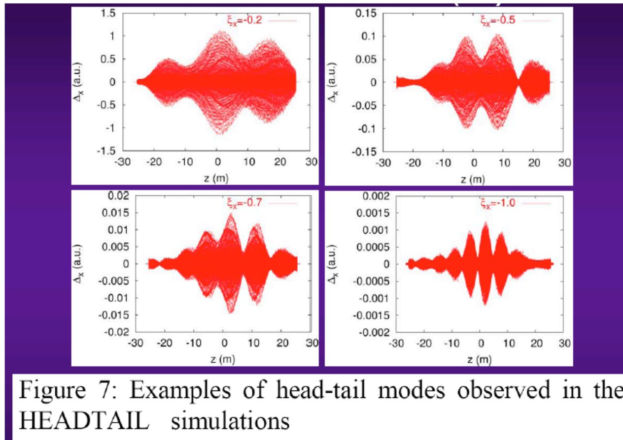
Figure 7: Examples of head-tail modes observed in the HEADTAIL simulations
