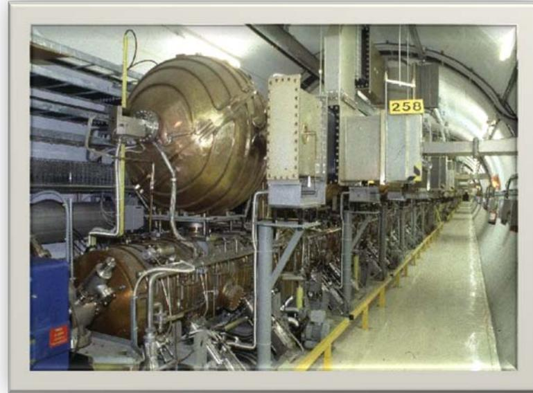
LEP normal-conducting Cu RF cavities,
