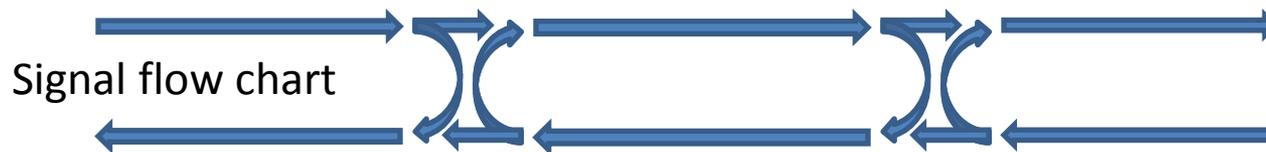
Reflections from notches lead to a superimposed standing wave pattern.
