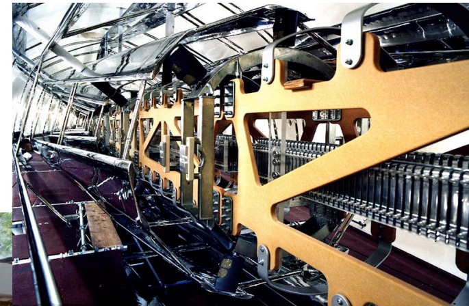
Vivitron, Strasbourg, inner structure of the acc. section
