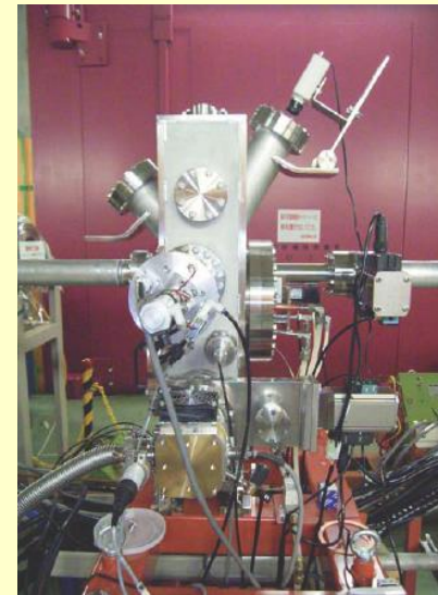
Rotating carbon disk stripper, thickness of the foil 100 \mu g/cm 2 , RIKEN
