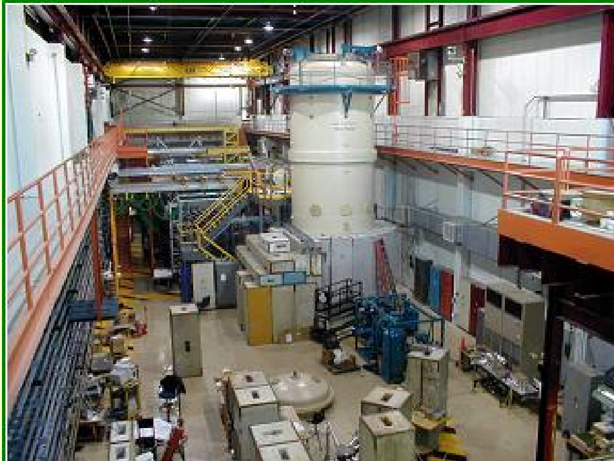
High energy electron cooling in FNAL's antiproton Recycler ring. 8 GeV antiprotons; 4.3 MeV/0.5 A electrons; Pelletron electrostatic electron accelerator.
