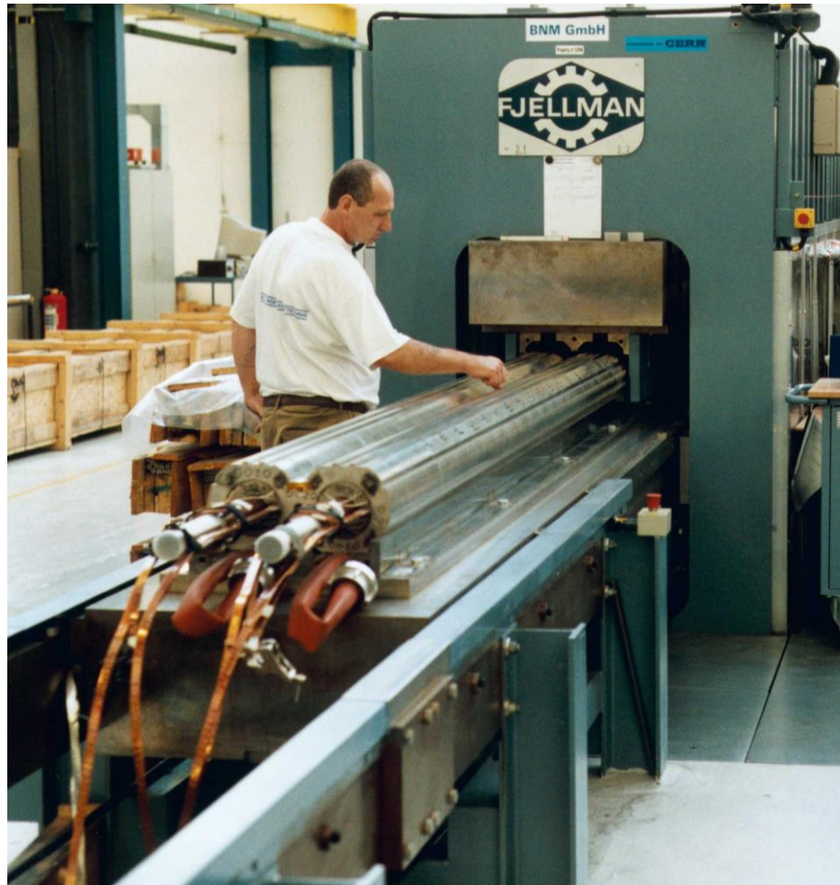
Collaring of a dipole magnet
